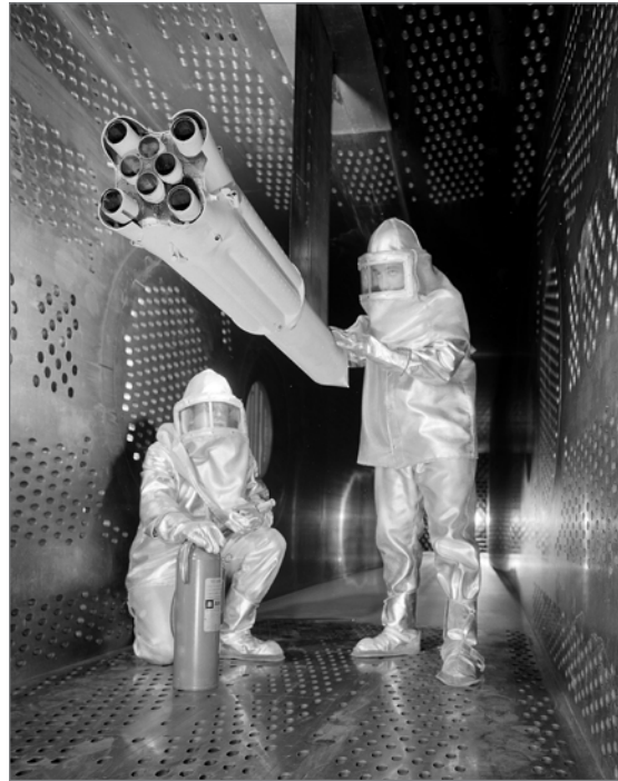
Saturn I booster tests take place in the 8- by 6-foot supersonic wind tunnel at NASA Lewis Research Center (now Glenn). (Image credit: NASA)
