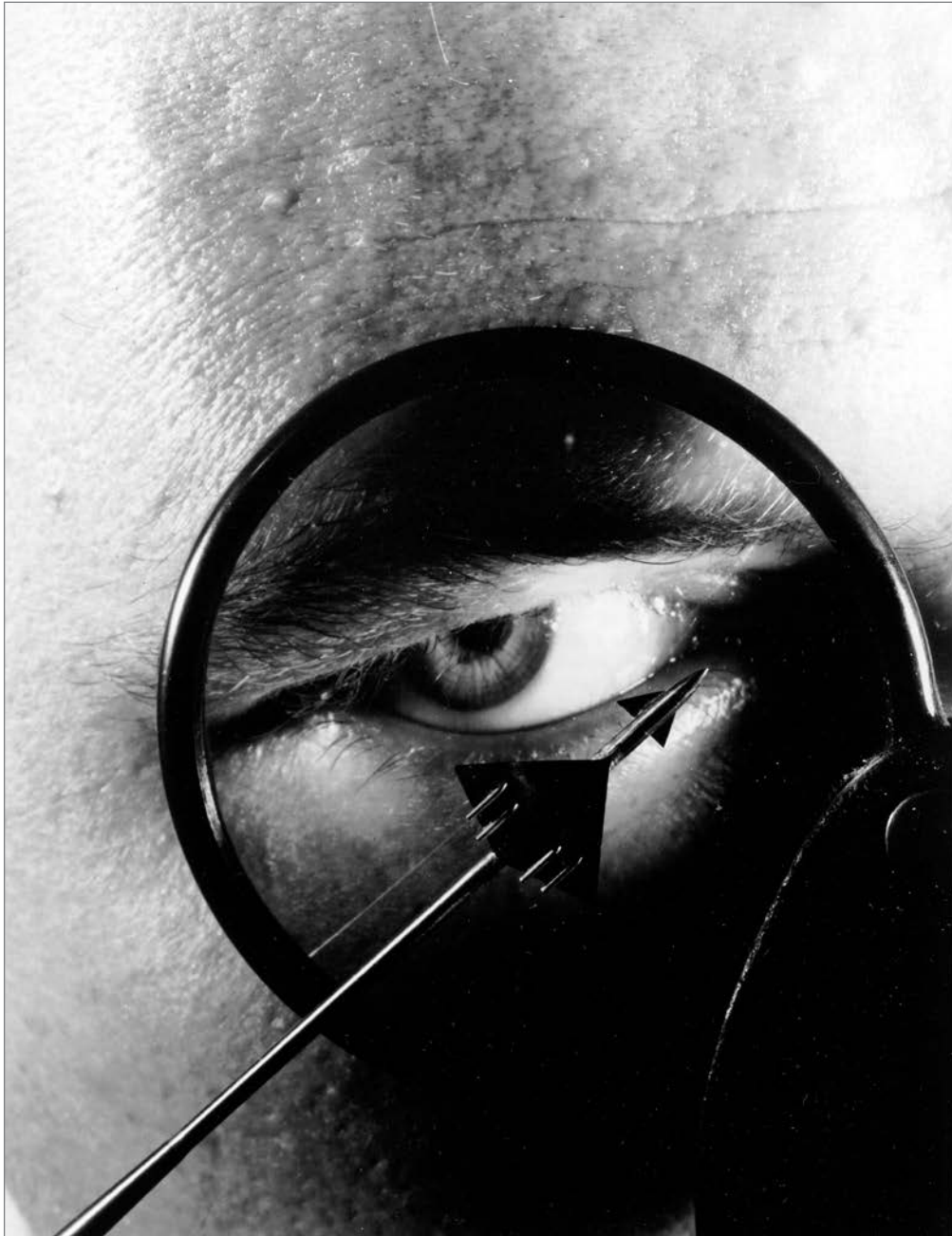
A 1-inch scale model of a typical supersonic airplane design is examined before being installed for sonic boom studies in the 4-foot supersonic tunnel at NASA's Langley Research Center ca. 1960. Pressure measurements are made in the tunnel up to 50 inches away from the model, simulating altitudes of up to 40,000 feet. (Photo credit: NASA)
