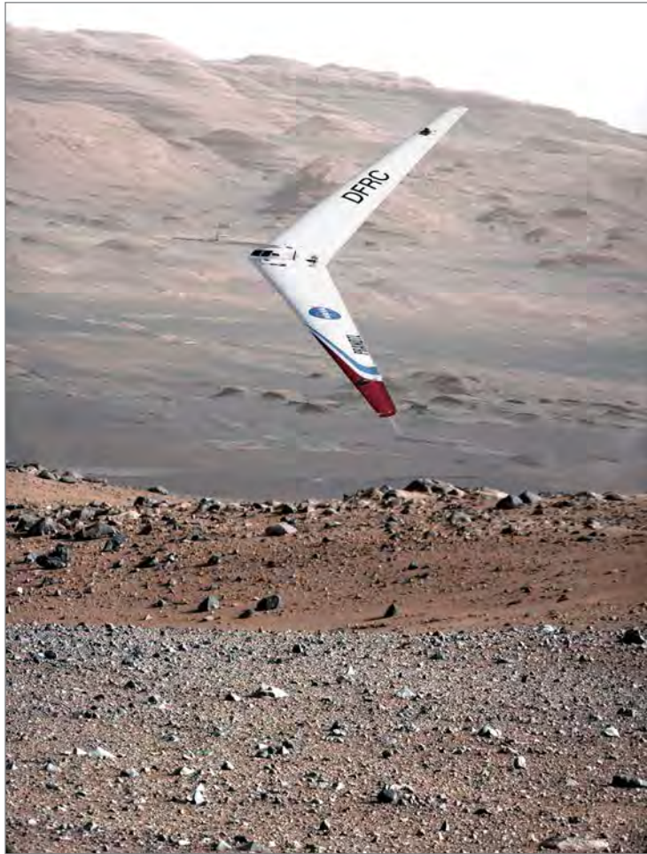
Shown is Prandtl-D, the second airframe, launched by a large bungee cord and flown by radio control.
