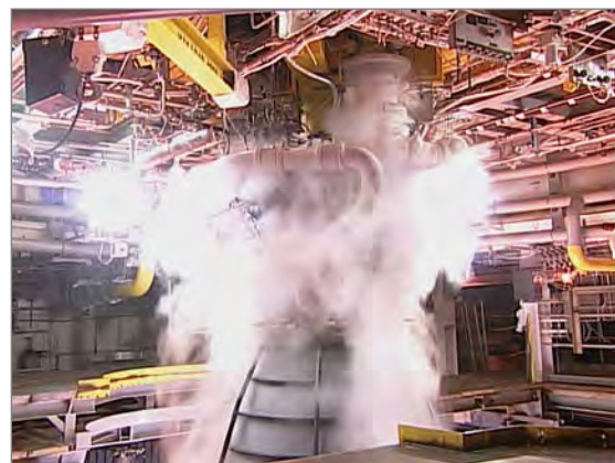
A close-up view shows the RS-25 engine during its recent hotfire test at Stennis.
