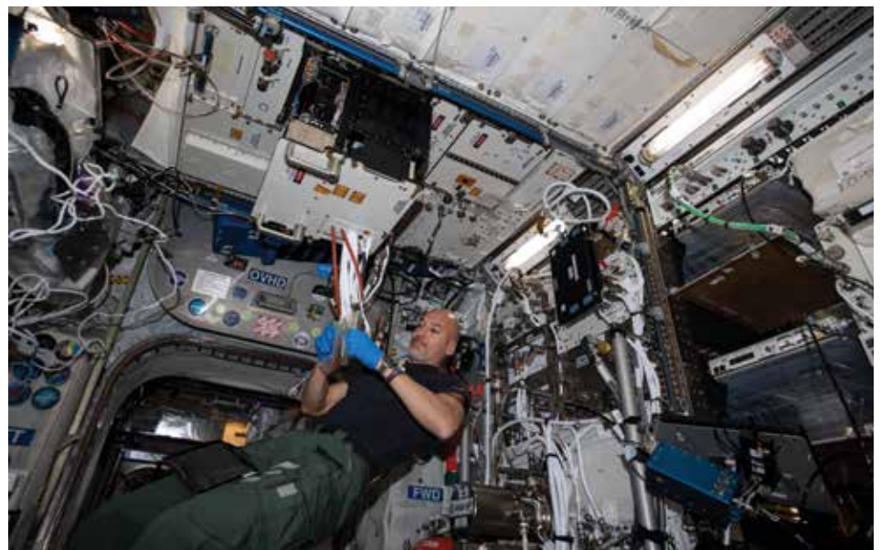
ESA astronaut Luca Parmitano installing the MultiScale Boiling Experiment Container (EC) in the Fluid Science Laboratory (FSL) in the Columbus Module. Credits: NASA/ESA
