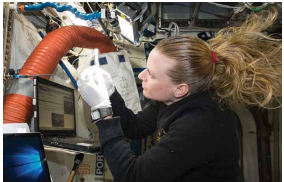
NASA astronaut Kate Rubins prepares for a run of the Biomolecule Sequencer experiment. It seeks to demonstrate, for the first time, that DNA sequencing is feasible in an orbiting spacecraft. A space-based DNA sequencer could identify microbes, diagnose diseases, help researchers understand crew member health, and has the potential to help detect DNA-based life elsewhere in the solar system. Credit: NASA
