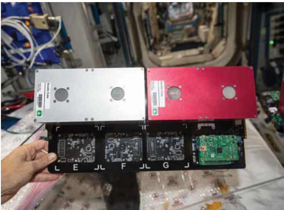
This image shows CubeLabs installed in Space Tango’s TangoLab facility, which provides a standardized platform and open architecture for these experimental modules for use in 3D tissue and cell cultures. Credit: NASA
