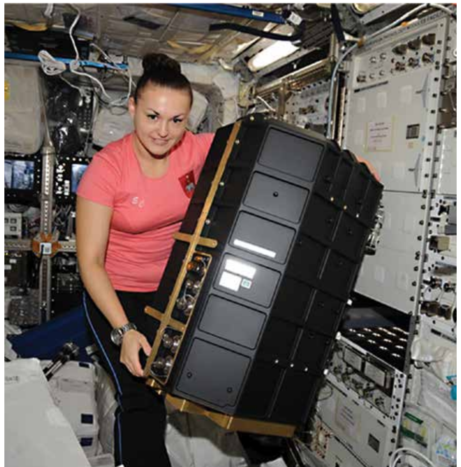
Russian cosmonaut Elena Serova installs the Plasma Kristall-4 apparatus in the Columbus module. The mass of the experimental part of the apparatus is over 100 kilograms (220 pounds) on Earth. Credits: ROSCOSMOS/ESA
