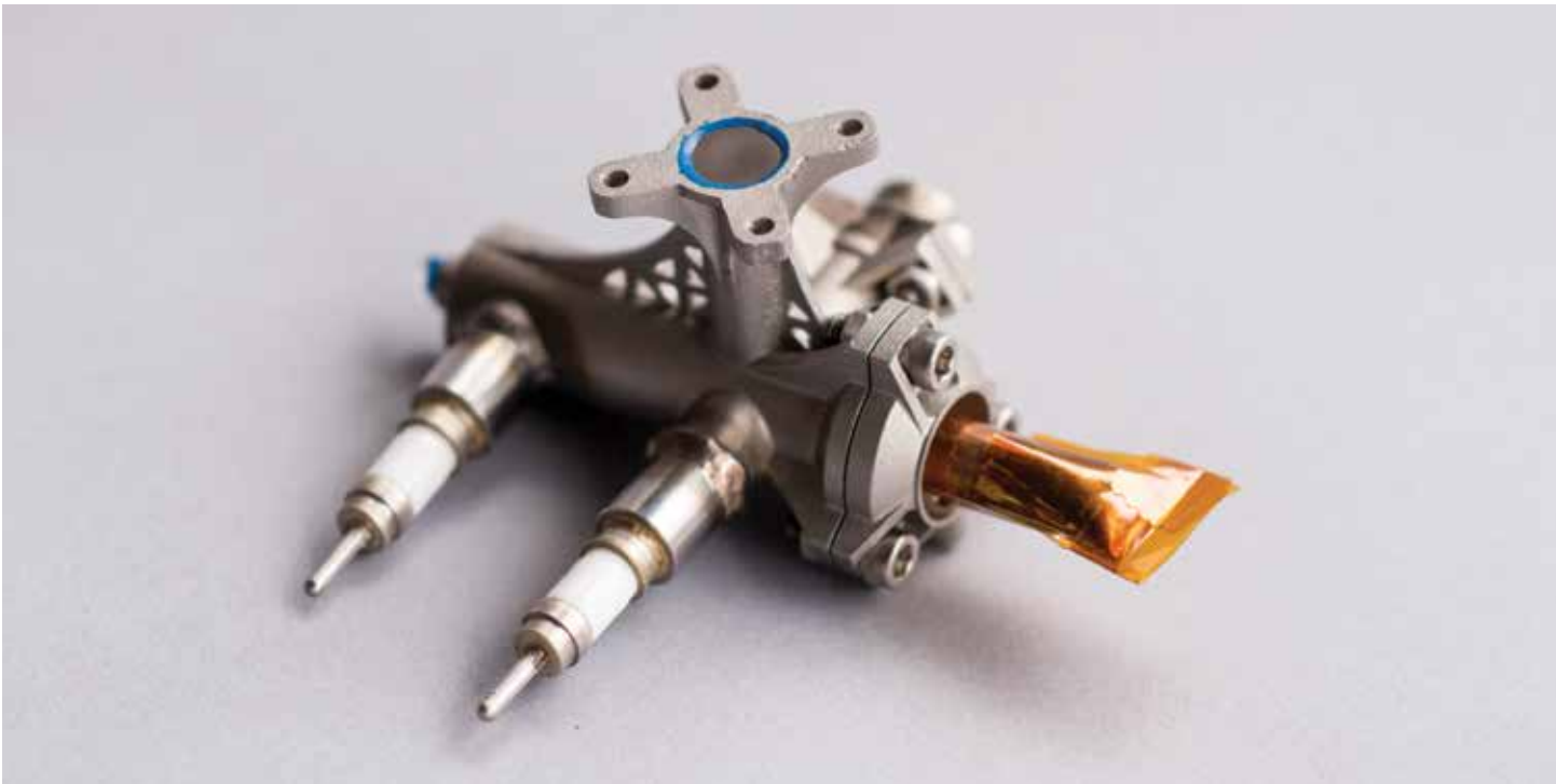
This miniaturized X-ray source was used to test the NICER payload and is now being used for developing new CT scan technology. The high-speed switching capability and miniature size make possible many new technologies, including X-ray-based communication, novel X-ray fluorescence and diffraction instruments for materials science, low and precise dose medical X-rays, and more. Credits: NASA/Goddard/Samantha Kilgore
