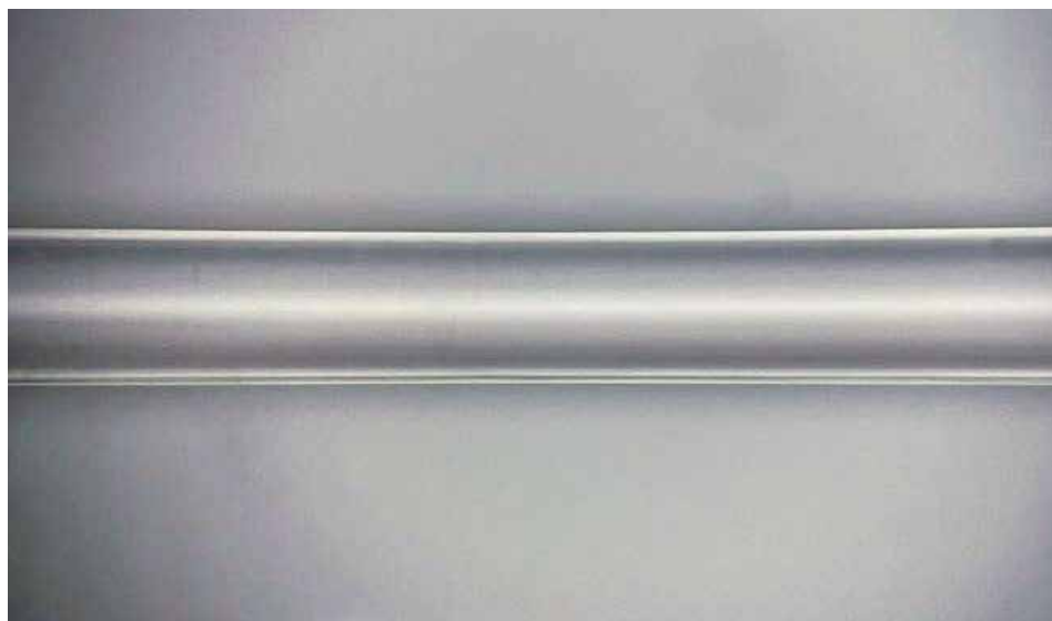
A microscopic image of a section of ZBLAN optical fiber produced by the second iteration of Fiber Optic Production aboard the International Space Station. Credit: Mercury Systems
