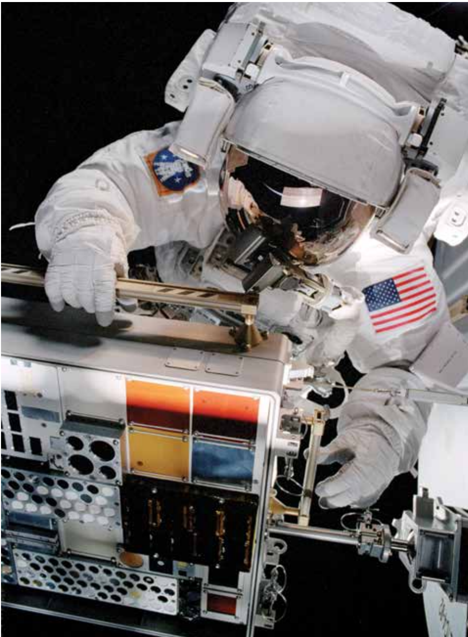
MISSE materials exposure device being installed on the space station for the first time in August 2001. The first externally mounted experiment conducted on the space station, MISSE-1 exposed 750 material samples to space for about 18 months. Credit: NASA
