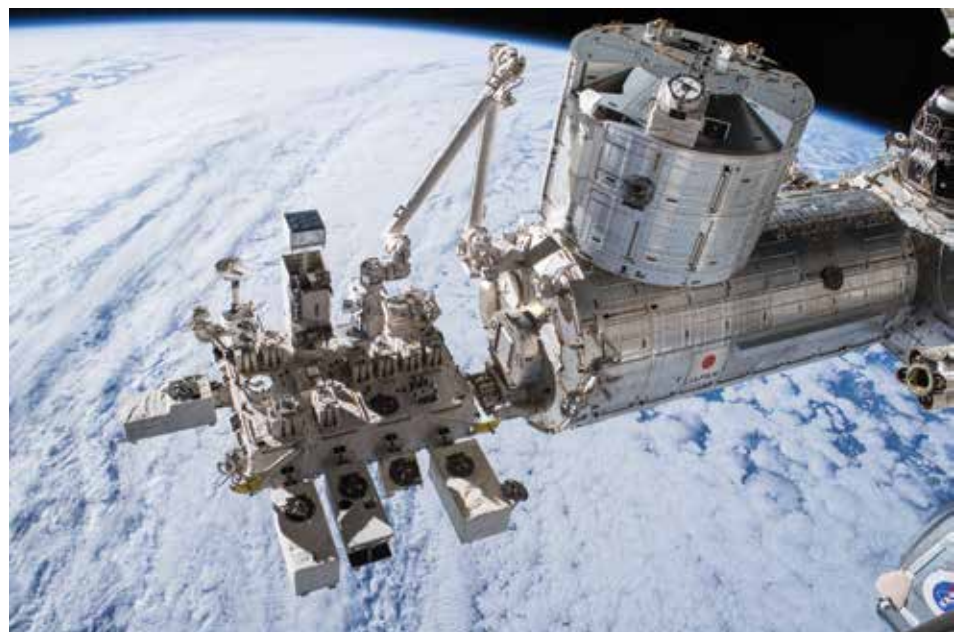
The suite of Earth-observing payloads attached to the Japanese Experiment Module is shown as the International Space Station orbits over the southern Pacific Ocean east of New Zealand in March 2018. Credit: NASA
