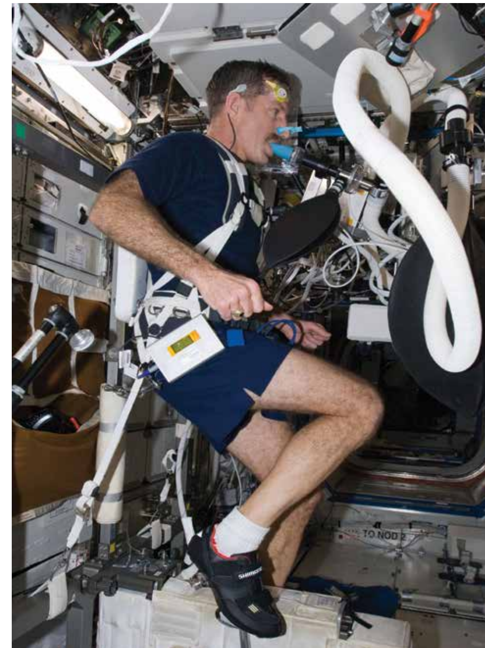
NASA astronaut Dan Burbank exercises on the Cycle Ergometer with Vibration Isolation and Stabilization (CEVIS) during a session of VO2max while Thermolab data are taken. Credit: NASA
