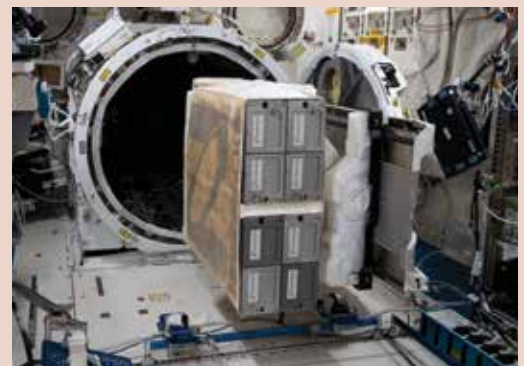
The NanoRack CubeSat Deployer (NRCSD)-16 investigation is shown aboard the space station prior to deployment of seven CubeSats that include Swiatowid. Credit: NASA
