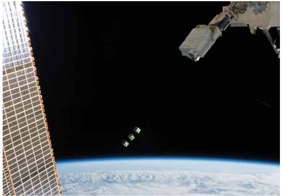
J-SSOD#11 deploys the Joint Global Multi Nation Birds, known as the BIRDS-3 Project. Credit: NASA
