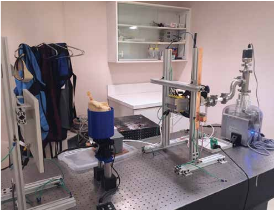
View of the experimental setup created by Dr. Raj Gupta's research team at Massachusetts General Hospital to image a pig lung to test the new CT scan method. The technology was developed using an X-ray source created for the NICER payload aboard the space station. Credit: Raj Gupta, Massachusetts General Hospital and Harvard Medical School
