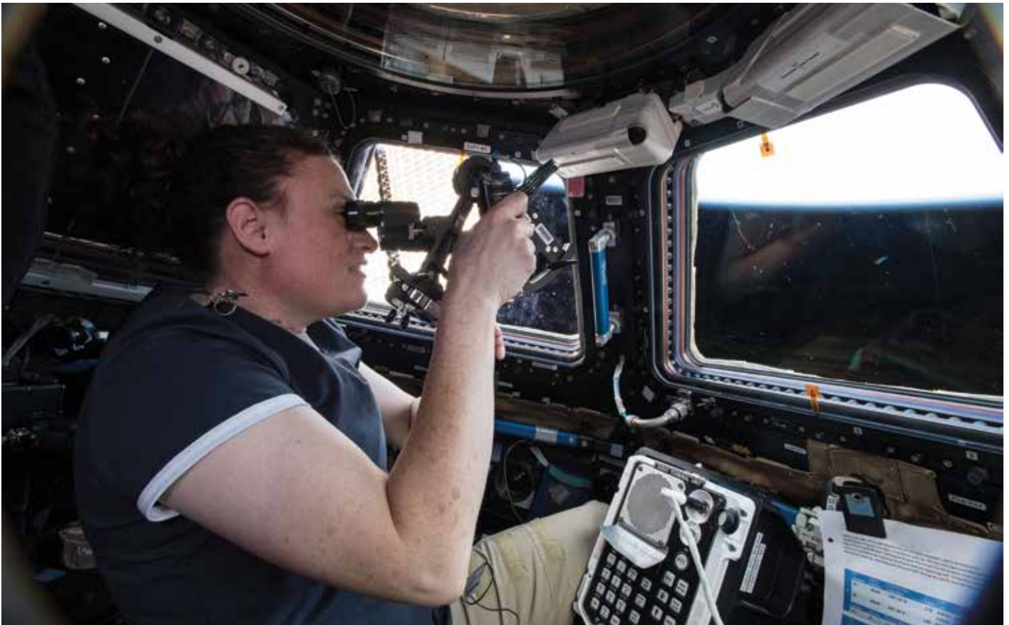
NASA astronaut Serena Auñón-Chancellor operating a sextant in the space station's cupola for the Sextant Navigation investigation. Credit: NASA
