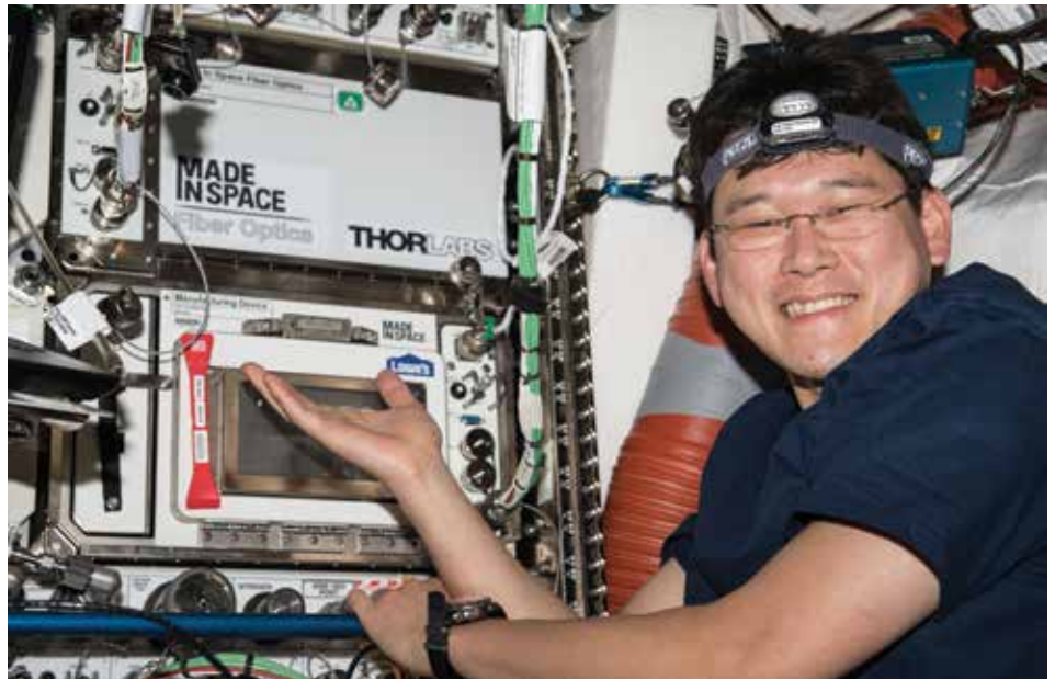
Japan Aerospace Exploration Agency (JAXA) astronaut Norishige Kanai poses for a photo with the installed Made in Space Fiber Optics Locker and the re-installed Additive Manufacturing Facility (AMF) manufacturing device. The Made In Space Fiber Optics investigation demonstrates the merits of manufacturing fiber optic filaments in microgravity. Credit: NASA
