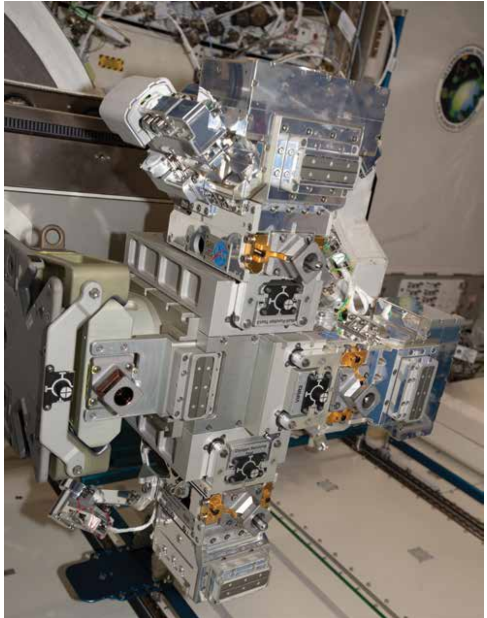
RRM3 hardware shown aboard the space station. This investigation demonstrates the first transfer and long-term storage of liquid methane, a cryogenic fluid, in microgravity. The ability to replenish and store cryogenic fluids, which can function as a fuel or coolant, can help enable long-duration journeys to destinations like the Moon and Mars. Credit: NASA
