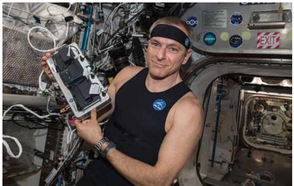
Canadian Space Agency astronaut David Saint-Jacques testing the Bio-Monitor, wearable technology designed to measure and record astronauts' vital signs. Credits: CSA/NASA
