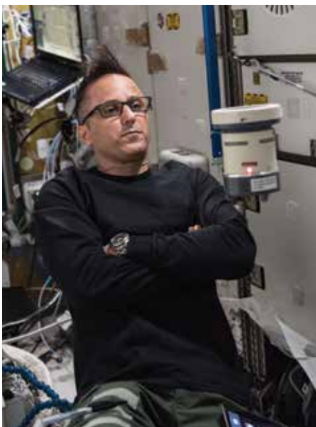
NASA astronaut Joe Acaba with one of the Microbial Air Samplers, devices that monitor microbes in the air of the space station. Credit: NASA
