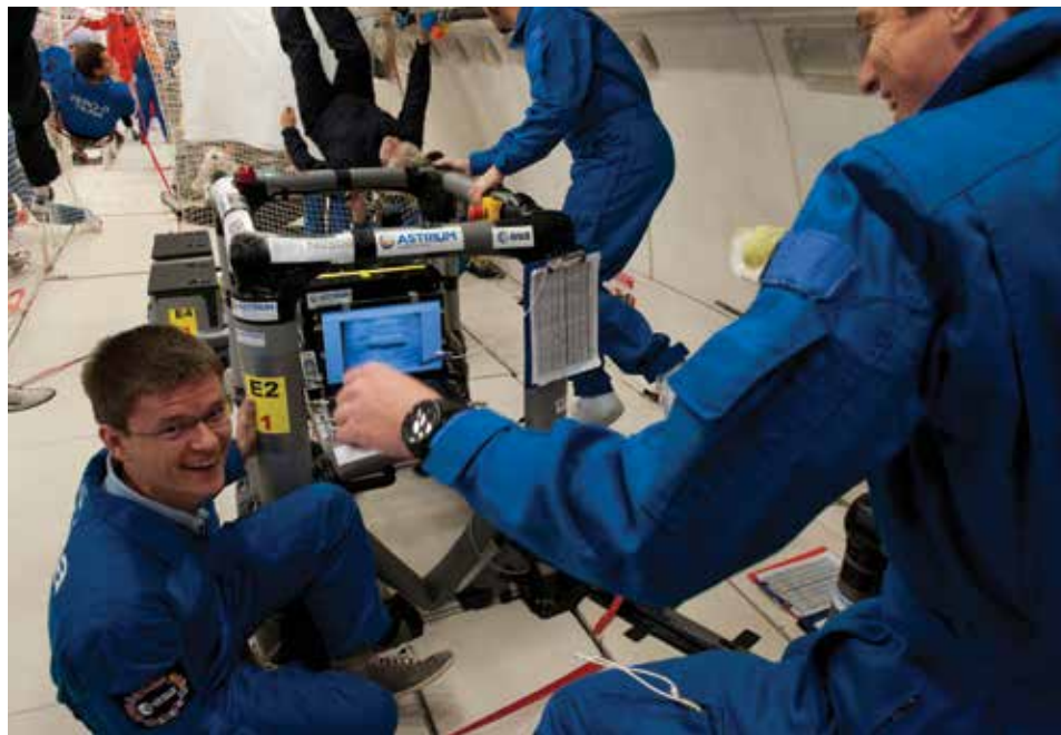
ESA (European Space Agency) scientist Sébastien Vincent-Bonnieu (left) performing zero-gravity foam experiments on a parabolic flight where short-term microgravity can be used to prepare and test experiments for the space station. Credit: ESA
