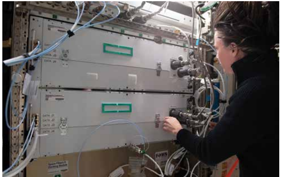
NASA astronaut Megan McArthur with Spaceborne Computer-2, which explores how commercial off-the-shelf computer systems can advance exploration by processing data significantly faster in space with edge computing and artificial intelligence capabilities. Credit: NASA
