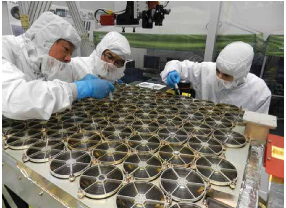
NICER team members apply epoxy to the X-ray concentrator mounts prior to launch. The epoxy held the optics assemblies fixed in position through the vibrations experienced during launch to the International Space Station. Credit: NASA
