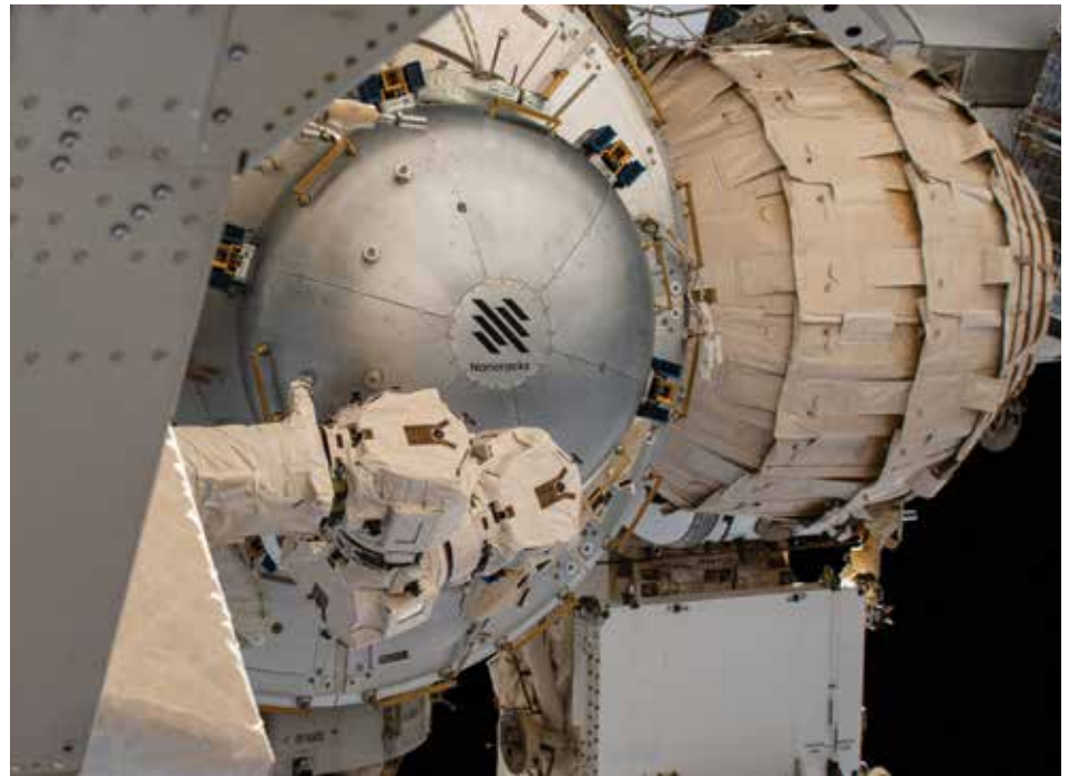
The Nanoracks Bishop airlock, shown here installed to the port side of the Tranquility module and still attached to the Canadarm2 robotic arm, increases the station’s capacity for private and public research and enables the release of larger satellites and the transfer of cargo inside and outside the station. Credit: NASA
