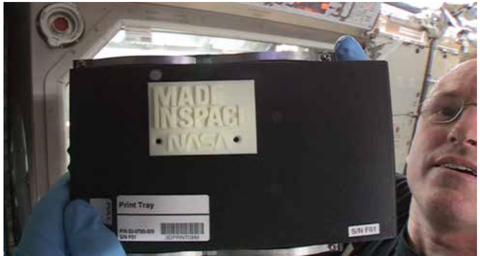
Commander Barry “Butch” Wilmore holds up the first object made in space with additive manufacturing or 3D printing. Credits: Made in Space/Redwire Space
