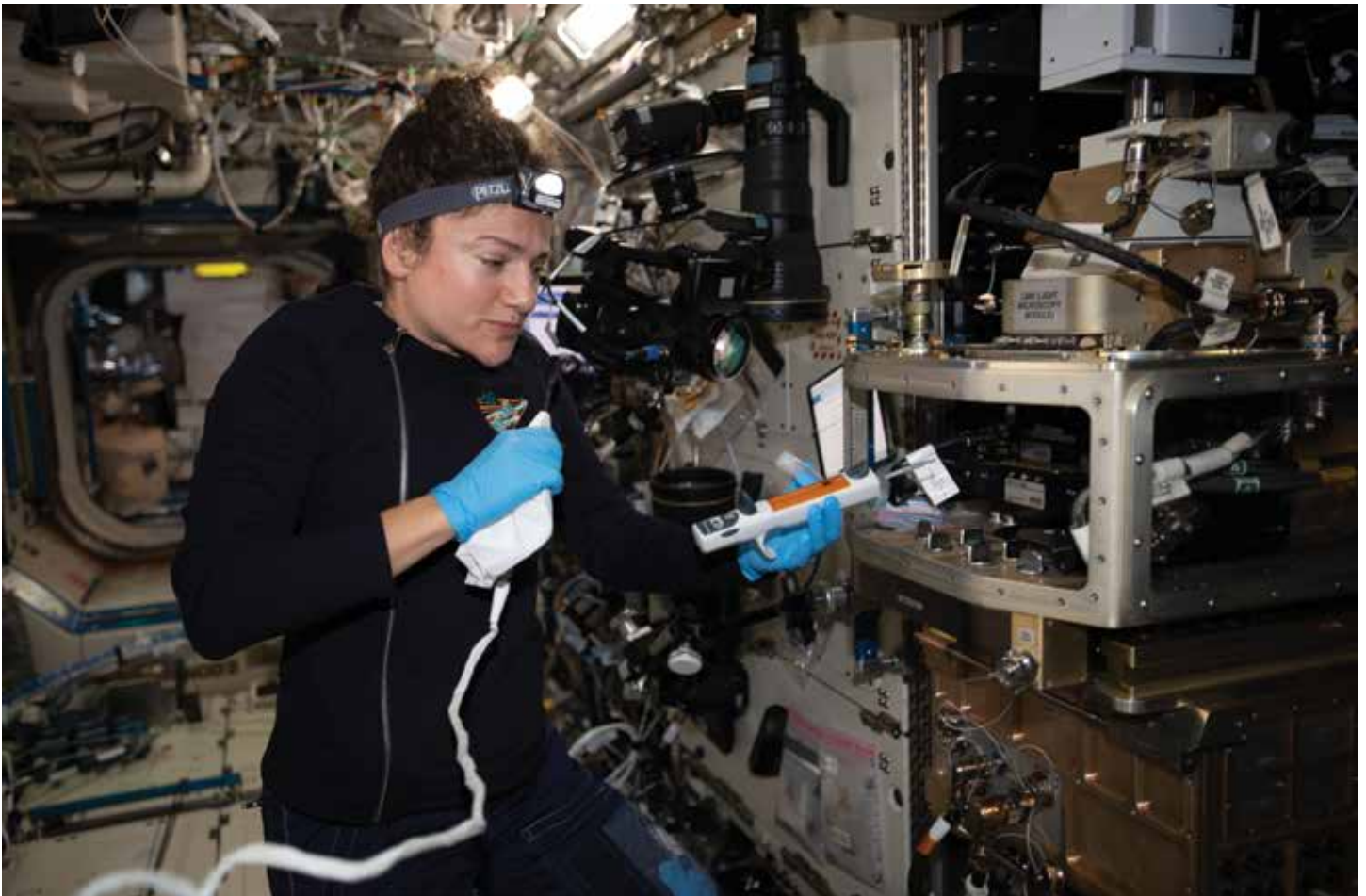
NASA astronaut Jessica Meir configures the Light Microscopy Module for the Advanced Colloids Experiment-Temperature-4 (ACE-T-4) study. ACE-T-4 examined the transition of an ordered crystal to a disordered glass to determine how increasing disorder affects structural and dynamic properties. Credit: NASA
