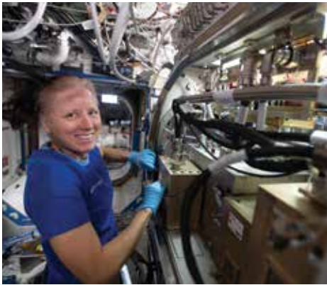
NASA astronaut Shannon Walker sets up Packed Bed Reactor Experiment (PBRE) hardware components. The PBRE study explores how liquids and gases behave together in a filtration packing material in microgravity, which may enable the design of more efficient, lightweight water recovery life support systems that use less energy on future space exploration missions. Credit: NASA
