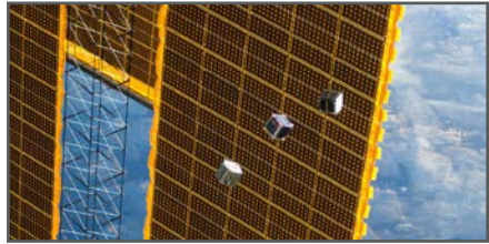
Figure 16. CubeSats deployed from the J-SSOD and photographed against the background of an ISS solar array.
