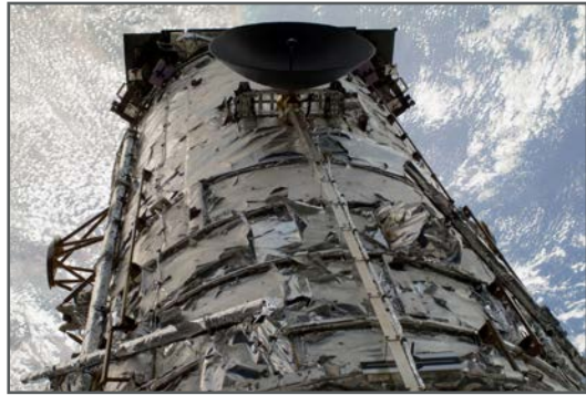
Severe degradation to the aluminized-Teflon outer layer of multilayer insulation after 19 years of space exposure (Yang and de Groh, 2010).
