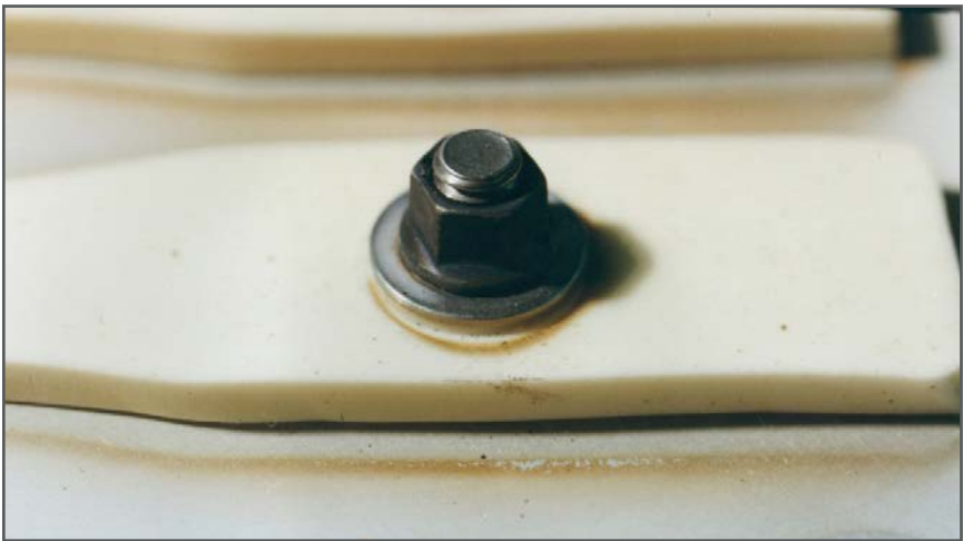
Figure 9. Postflight photograph shows a room temperature vulcanization sample from the Long Duration Exposure Facility A0171 experiment with deposited silicone contaminant on baseplate and sample. Also note oxidized silver fastener.
