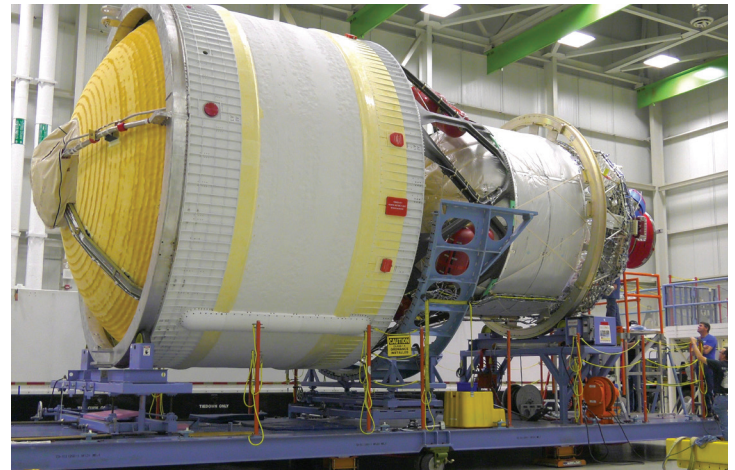
The ICPS is a single-engine liquid hydrogen/liquid oxygen stage based on the Delta Cryogenic Second Stage from ULA that produces 24,750 lbs. (110 t) of thrust and performs the TLI burn to send Orion toward the Moon.
