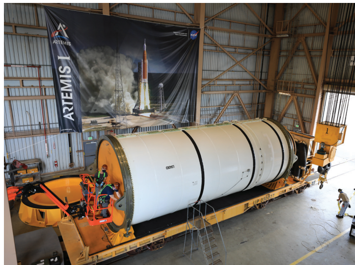
Artemis I booster motors travel by rail, left, from prime contractor Northrop Grumman facilities in Utah to Kennedy. Right, motor segments are offloaded, inspected, and stored at Kennedy's RPSF before transport to the Vehicle Assembly Building for stacking on the mobile launcher.
