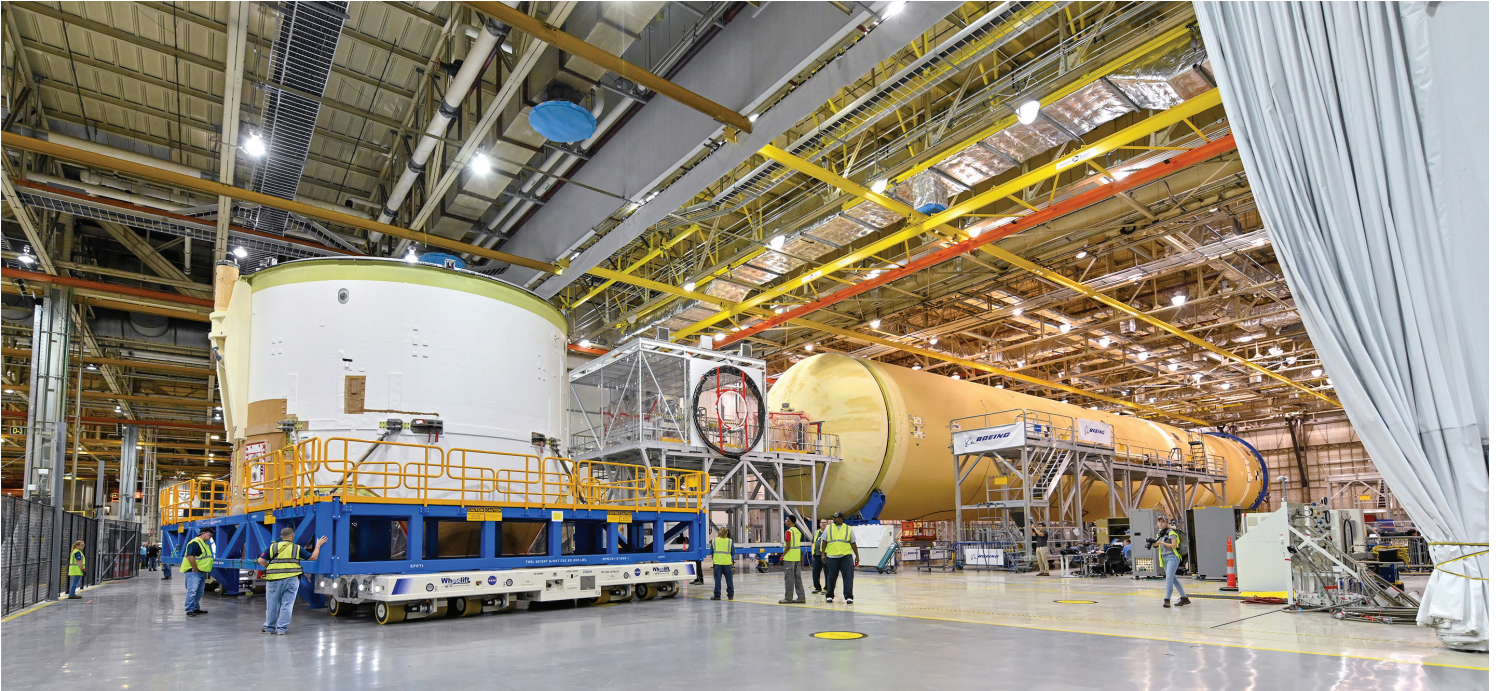
The SLS Artemis I engine section, left, and liquid hydrogen tank, right, at Michoud prior to integration.
