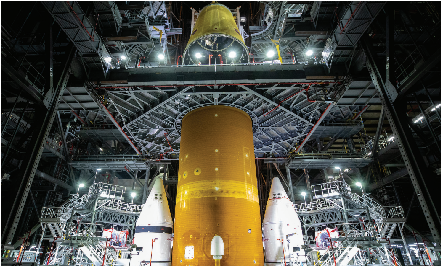
The SLS gets its signature orange color when its spray-on foam insulation darkens with exposure to sunlight. The core stage below the work platform was exposed to months of sunlight during Green Run testing at Stennis, while the launch vehicle stage adapter being lowered into place above the platform has been stored indoors since its completion.
