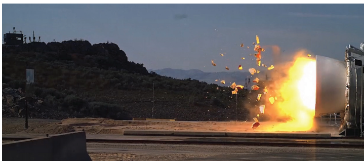
Close-up view of the throat plug break up and expulsion from the nozzle during ignition of the Qualification Motor 2 full-scale test firing in Utah.
