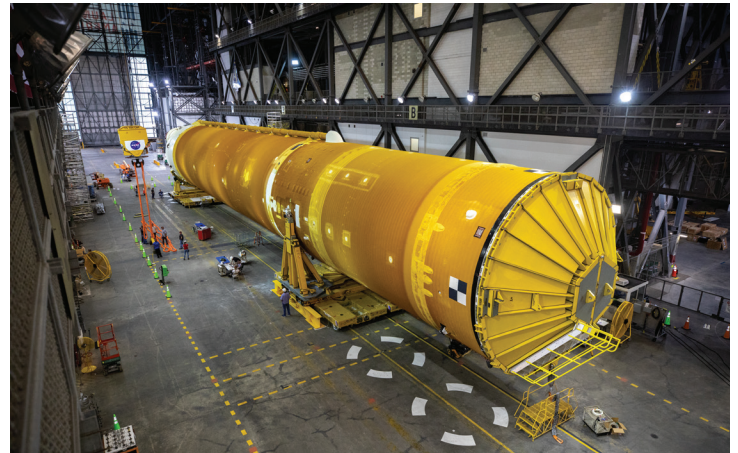
The Artemis I core stage waits in the Vehicle Assembly Building transfer aisle before stacking on the mobile launcher.
