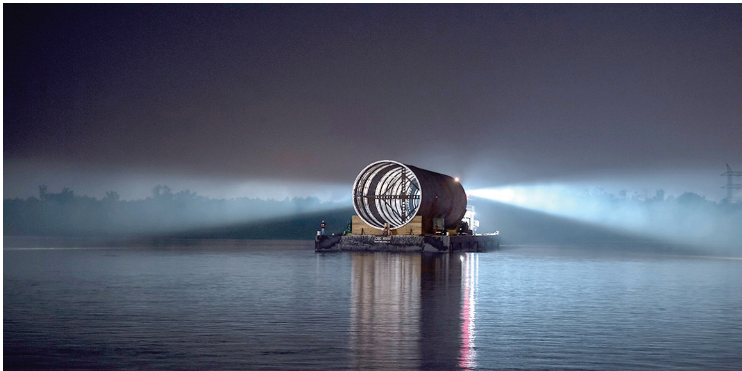
The core stage pathfinder mimics the structure of the SLS core stage, providing transportation, logistics, and lifting crews with the opportunity to rehearse with full-scale hardware before handling one-of-a-kind flight hardware.
