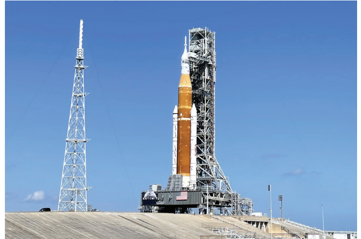
Stacked Artemis I rocket, consisting of SLS and Orion, on the mobile launcher.
