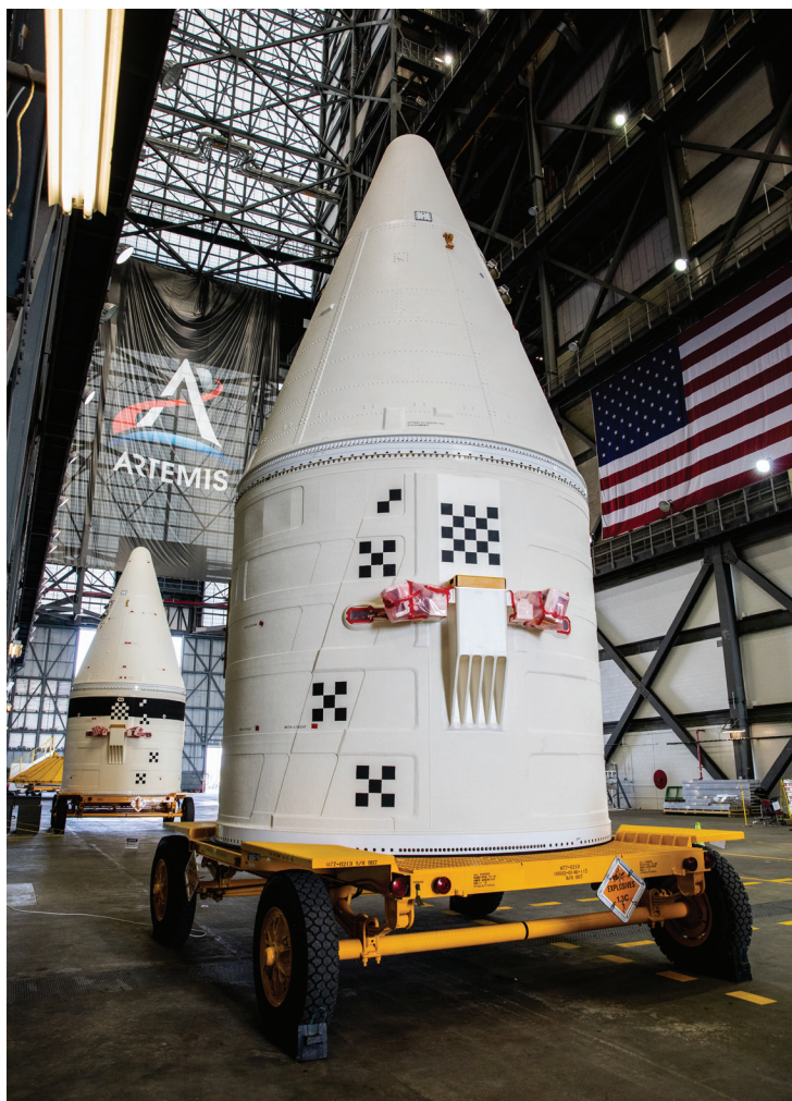
The forward assemblies for the SLS solid rocket boosters include aerodynamic nose cones, frustums, and forward skirts containing avionics.
