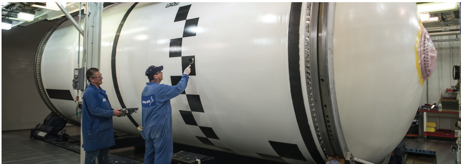
Technicians with lead solid rocket boosters contractor Northrop Grumman paint photogrammetric markings on one segment of an SLS solid rocket motor. The black-and-white targets painted on each element of the rocket provide targets for cameras, which then use those positions compared with fixed positions on the ground and on the mobile launcher to precisely locate SLS in space.
