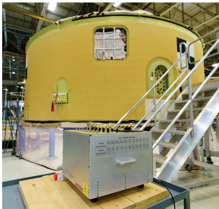
The core stage forward skirt contains the flight computers for the Block 1 SLS rocket.
