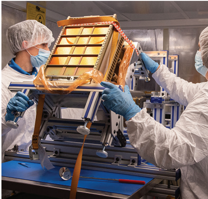
The NEA Scout CubeSat payload is integrated into its dispenser prior to the Artemis I flight.
