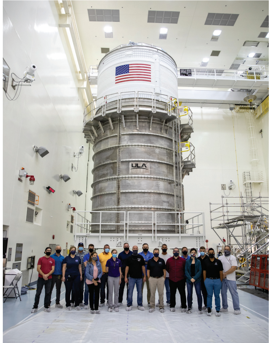
ULA supplies the ICPS, which is based on the Delta Cryogenic Second Stage, for the SLS Block 1 rocket.
