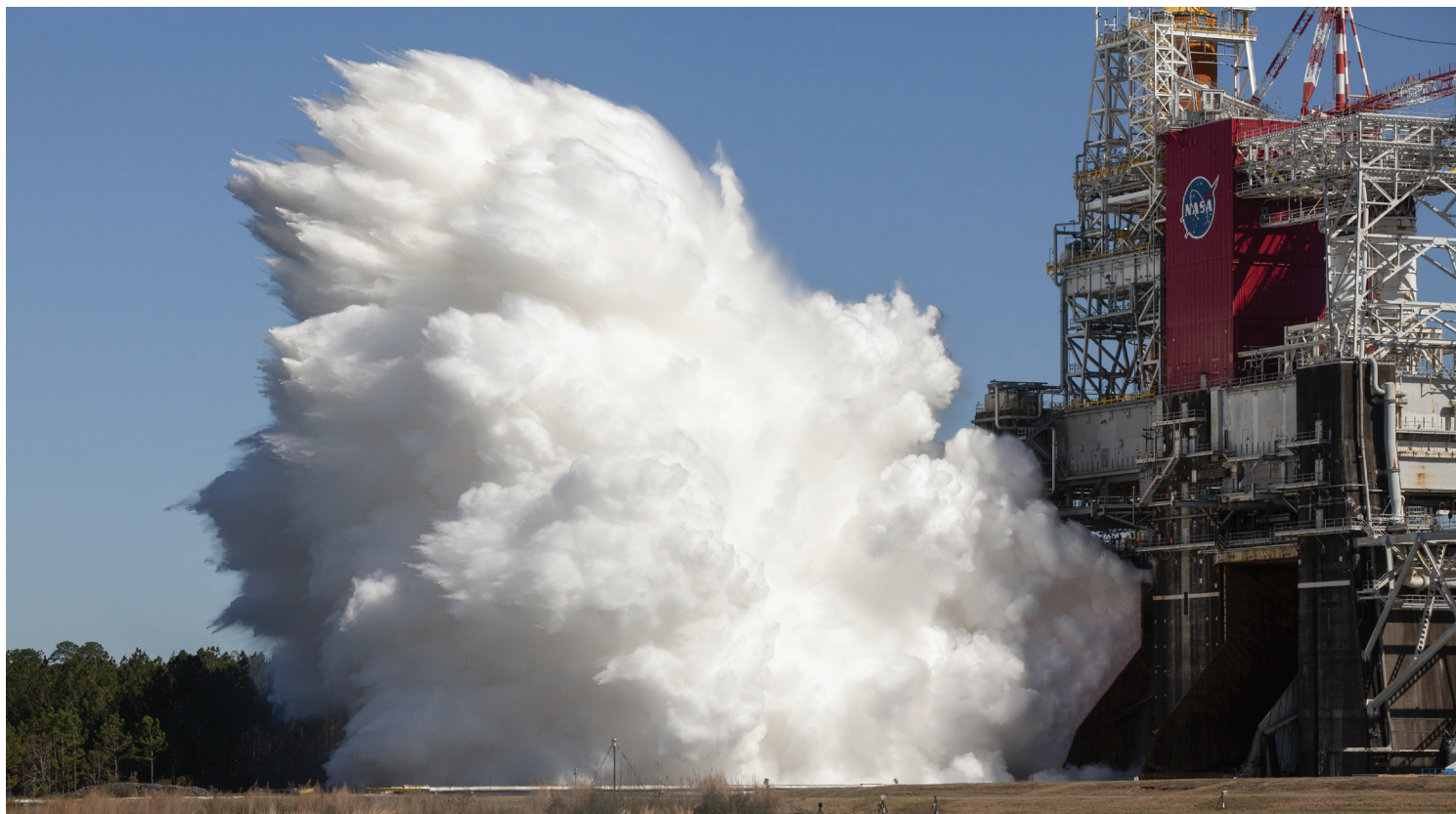
Eight major "Green Run" tests at Stennis of the Artemis I core stage and RS-25 engines culminated in a full-duration hot firing, the largest test of liquid-fueled engines since the Apollo Program.
