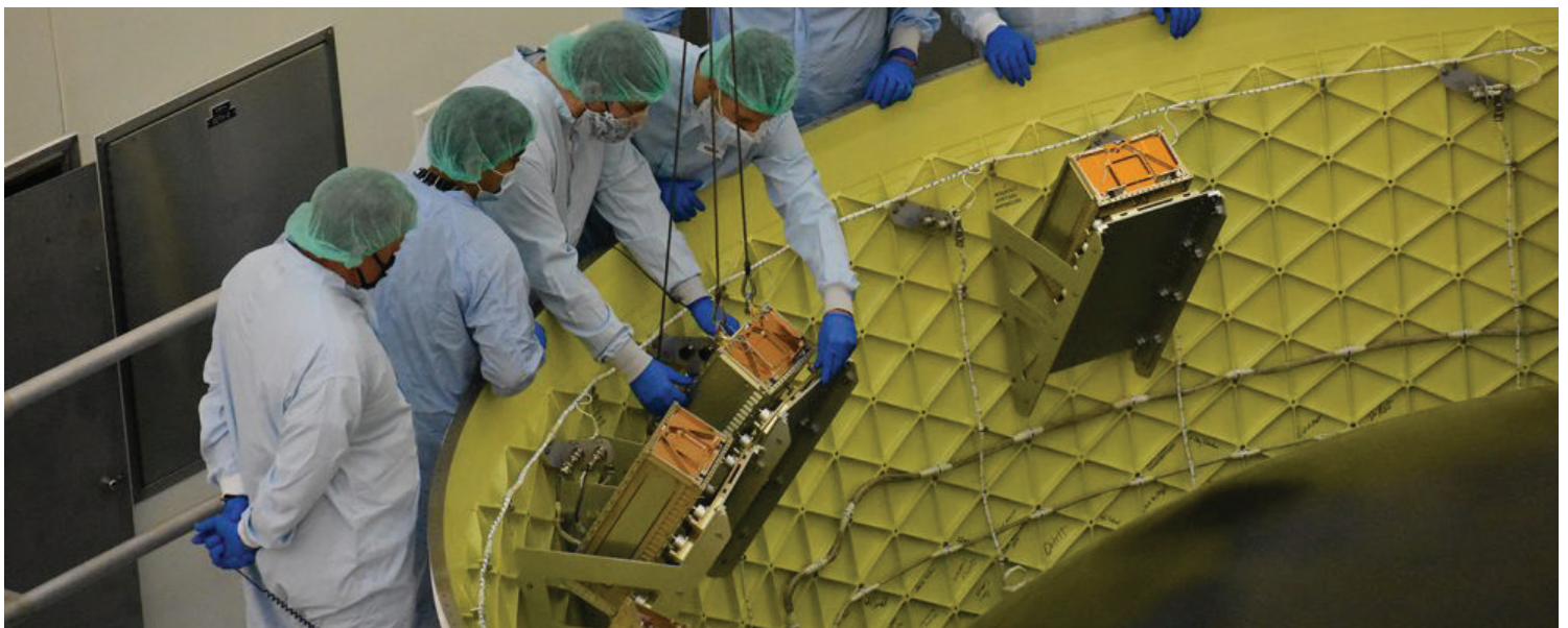
The Jacobs team at NASA Kennedy installing the last of 10 CubeSats in the SLS rocket's Orion stage adapter. BioSentinel, the final CubeSat to be loaded, will study how radiation affects living organisms in deep space.
