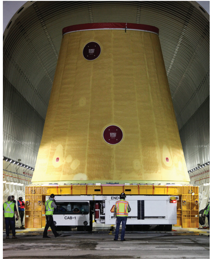
The launch vehicle stage adapter adapter partially encloses the ICPS and contains the pyrotechnic system to separate itself and the core stage from the ICPS and Orion.
