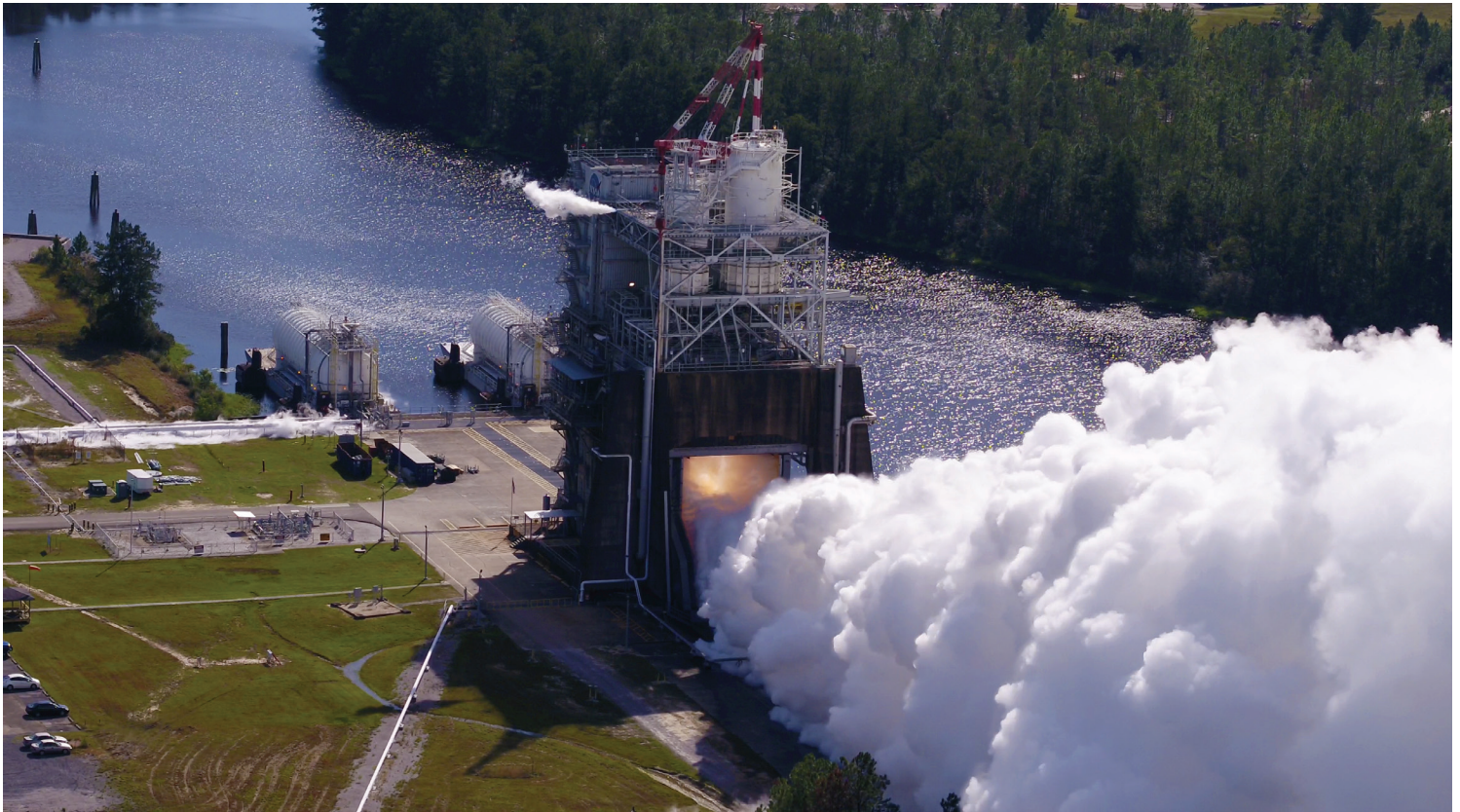
RS-25 hot fire testing at NASA's Stennis Space Center in Bay St. Louis, Mississippi, helped qualify engines to extreme SLS environments.
