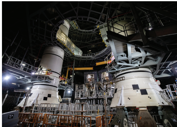
The solid rocket boosters' aft assembly includes the aft skirts with thrust vector control system inside that helps steer SLS during ascent. The entire weight of the SLS rocket goes through the aft skirt structures.
