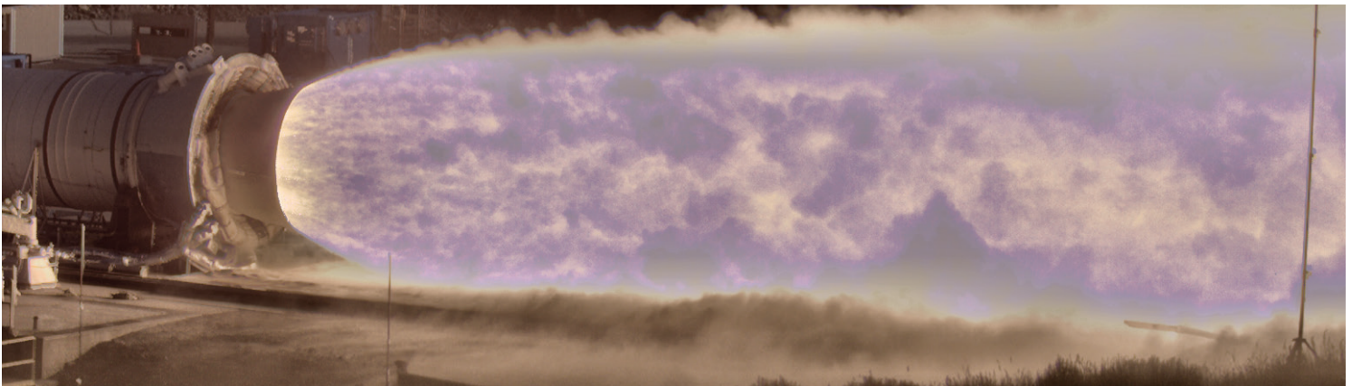
Boosters lead contractor Northrop Grumman and NASA hot-fired several full-scale solid rocket motors to help qualify them for the SLS Program.
