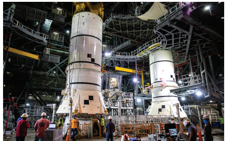
Artemis I booster aft assemblies ready for stacking in Kennedy Vehicle Assembly Building.
