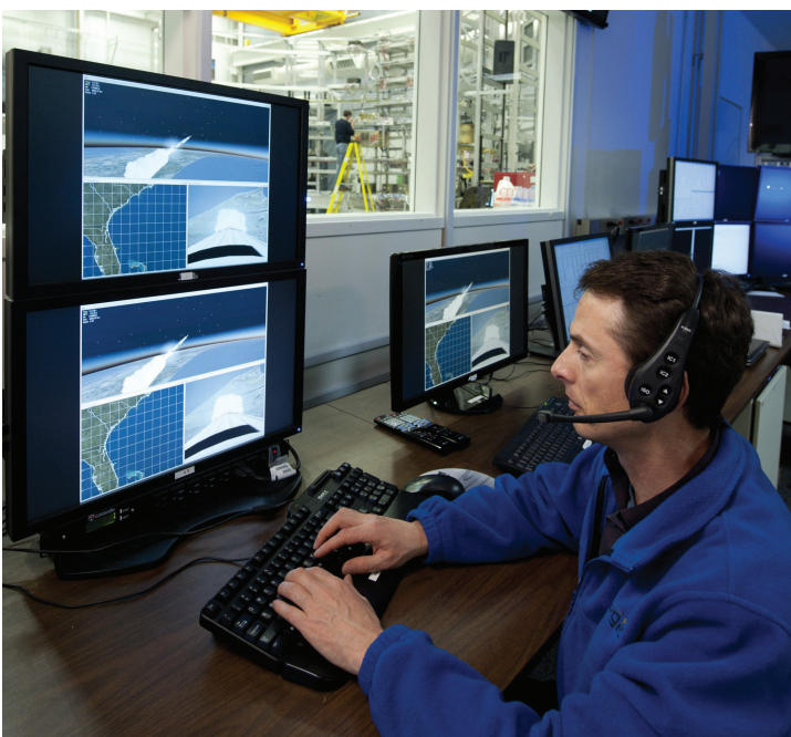
Marshall's Systems Integration Lab has the capabilities to allow the software team to fly thousands of virtual launches in a simulated environment that included wind, weather, and Earth's rotation.
