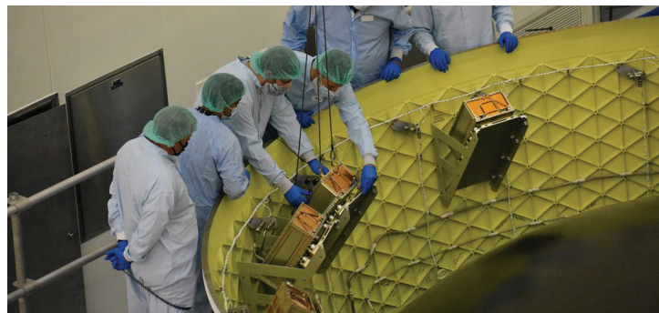
The Artemis I Orion stage adapter with mounting brackets for secondary payloads.
