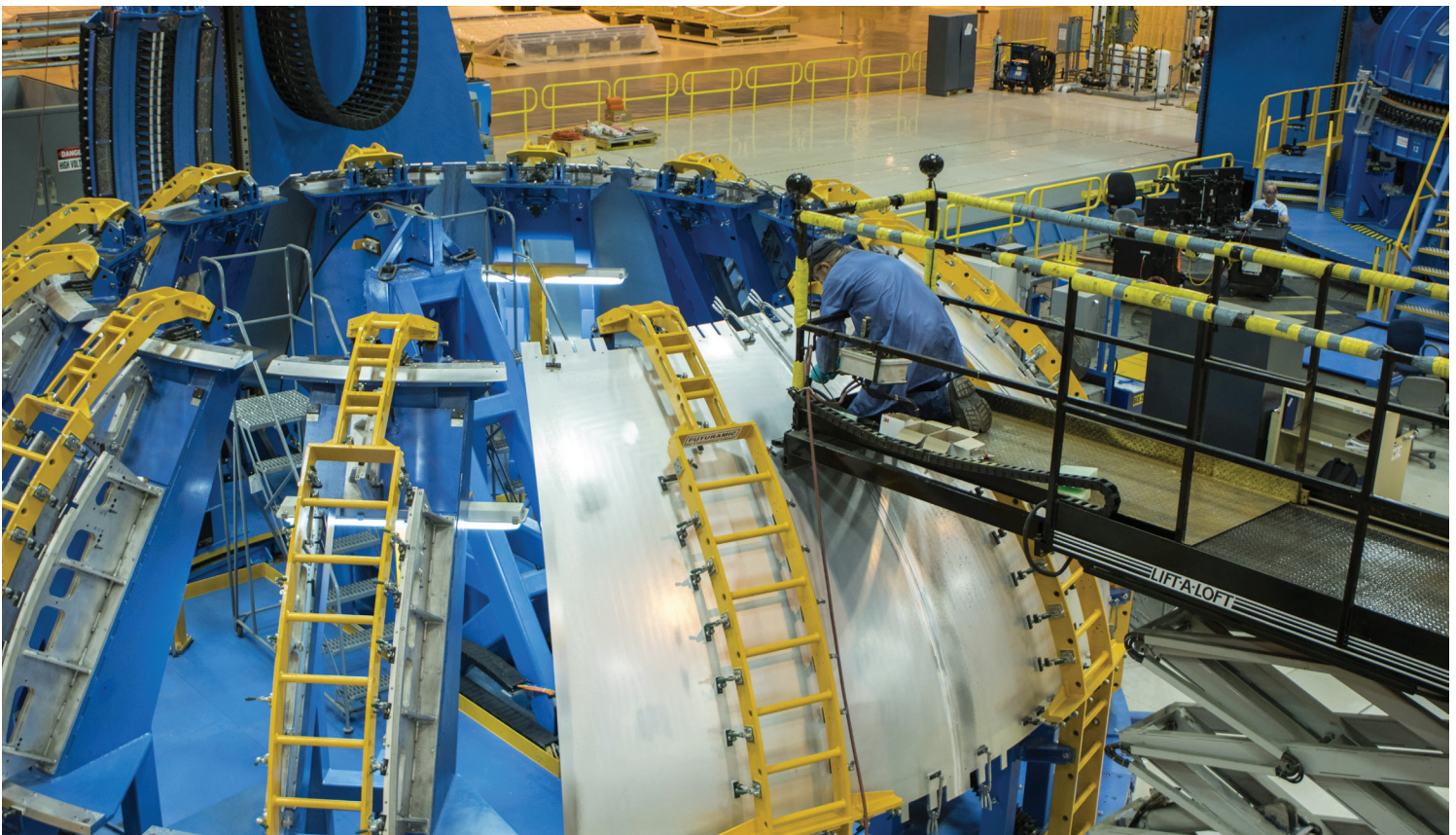
The gore weld tool at Michoud is used to weld domes for the SLS core stage propellant tanks.
