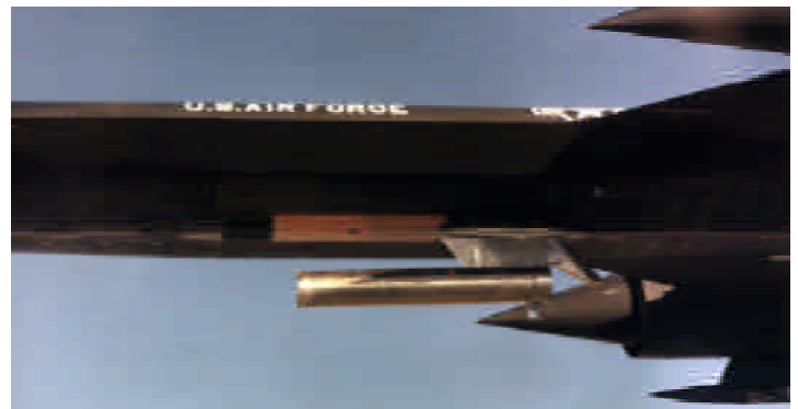
YF-12A 06935 with insulated hollow cylinder used on the Cold Wall Experiment. (NASA photo ECN-4777)
