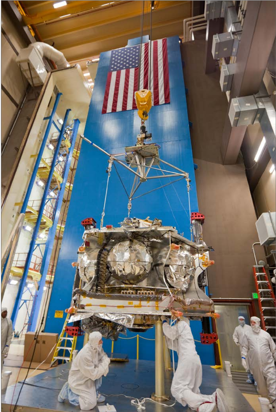
Preparing Juno for acoustical testing. (NASA/JPL-Caltech/LMSS: PIA13718)
