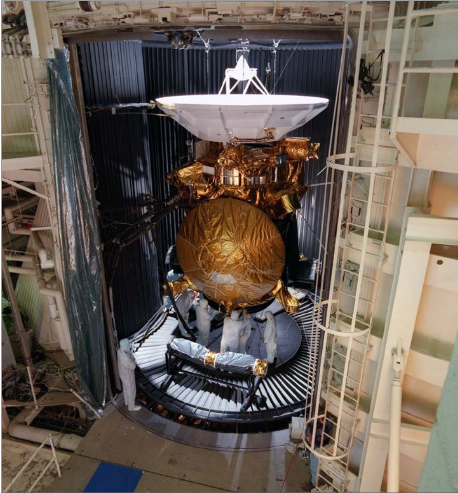
The newly assembled Cassini Saturn probe undergoes vibration and thermal testing at the JPL facilities in Pasadena, California. (NASA: p48313bc)
