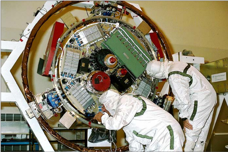
Jet Propulsion Laboratory (JPL) workers examine and repair the Huygens probe after damage was discovered during testing. (NASA: KSC-97PC-1392)
