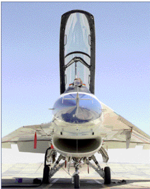
Front of F-16XL-2 showing wings as modified for flight research. NASA photo EC95-43267-2
