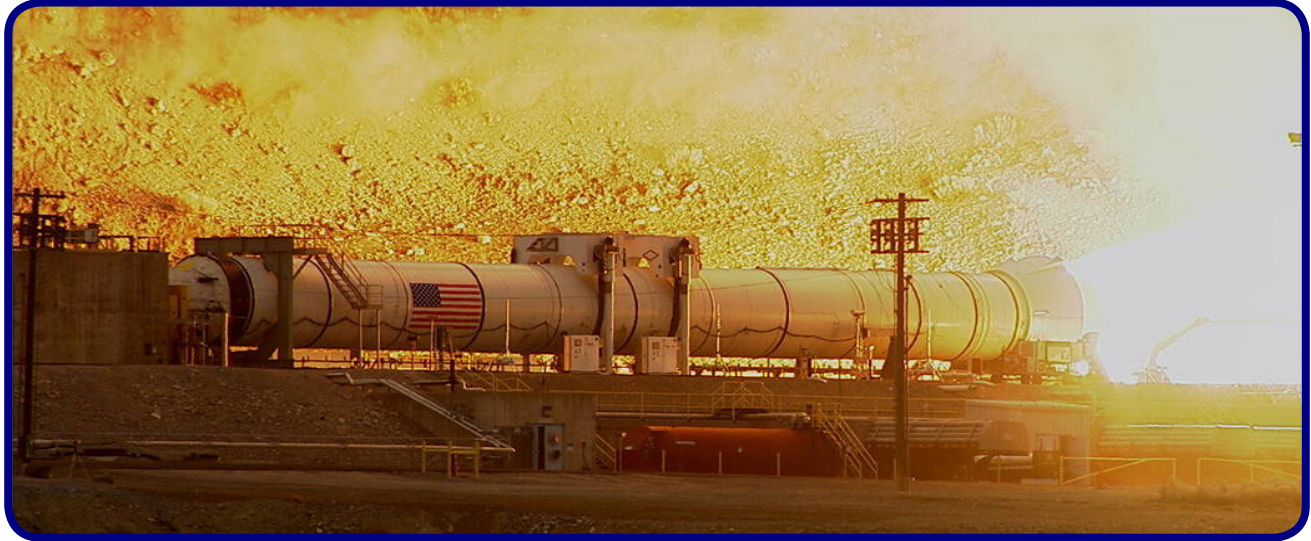
Image Caption: The first test fire of the booster for NASA's SLS rocket. (Credit: NASA)
