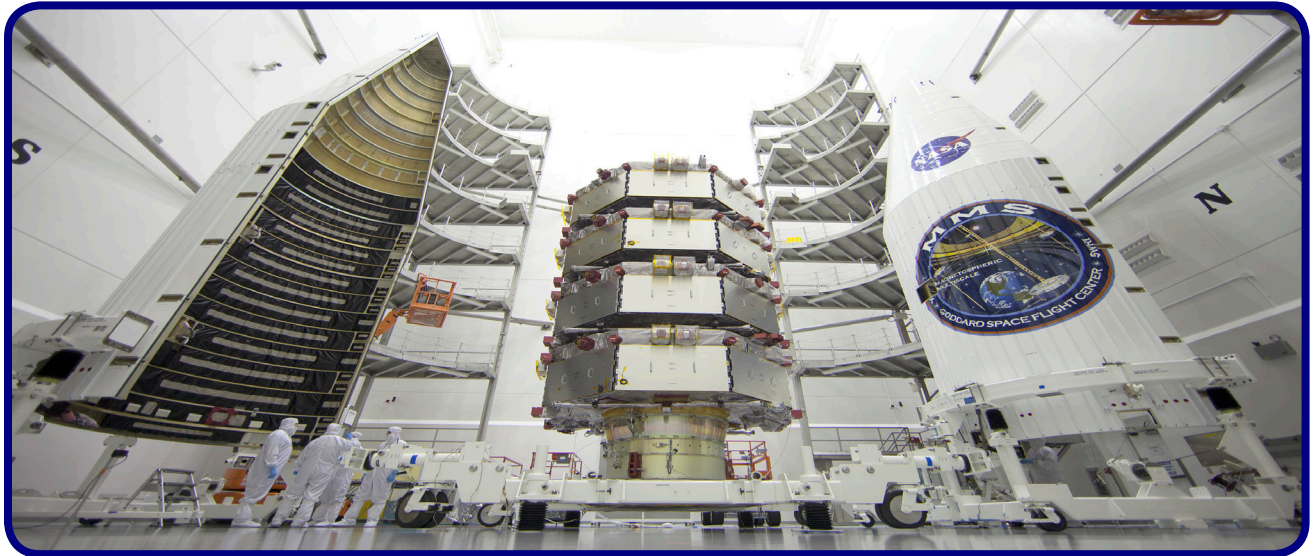
Image Caption: The four MMS observatories were processed for launch in a clean room at the Astrotech Space Operations facility in Titusville, Florida. (Credit: NASA/Ben Smegelsky)
