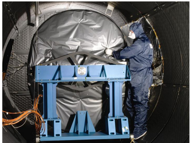
The Mid-Infrared Instrument, a component of NASA James Webb Space Telescope, undergoes testing. Credit: NASA
