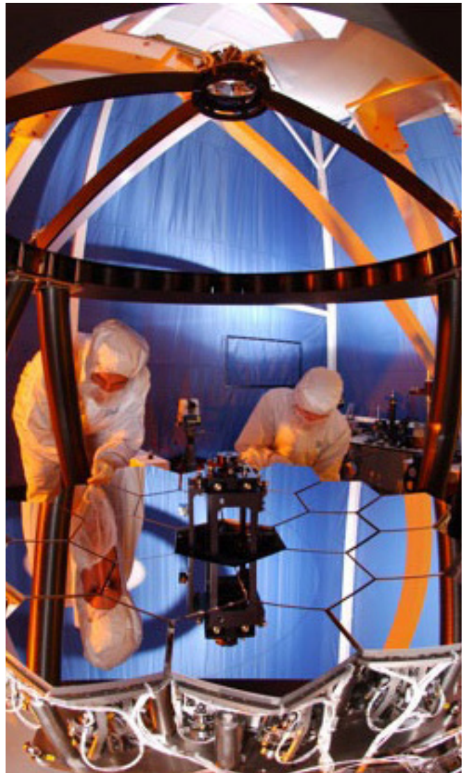
Engineers test the Wavefront Sensing and Control testbed for the James Webb Space Telescope. The test is performed on a 1/6 scale model of the JWST mirrors. Credit: NASA/Northrop Grumman/Ball Aerospace
