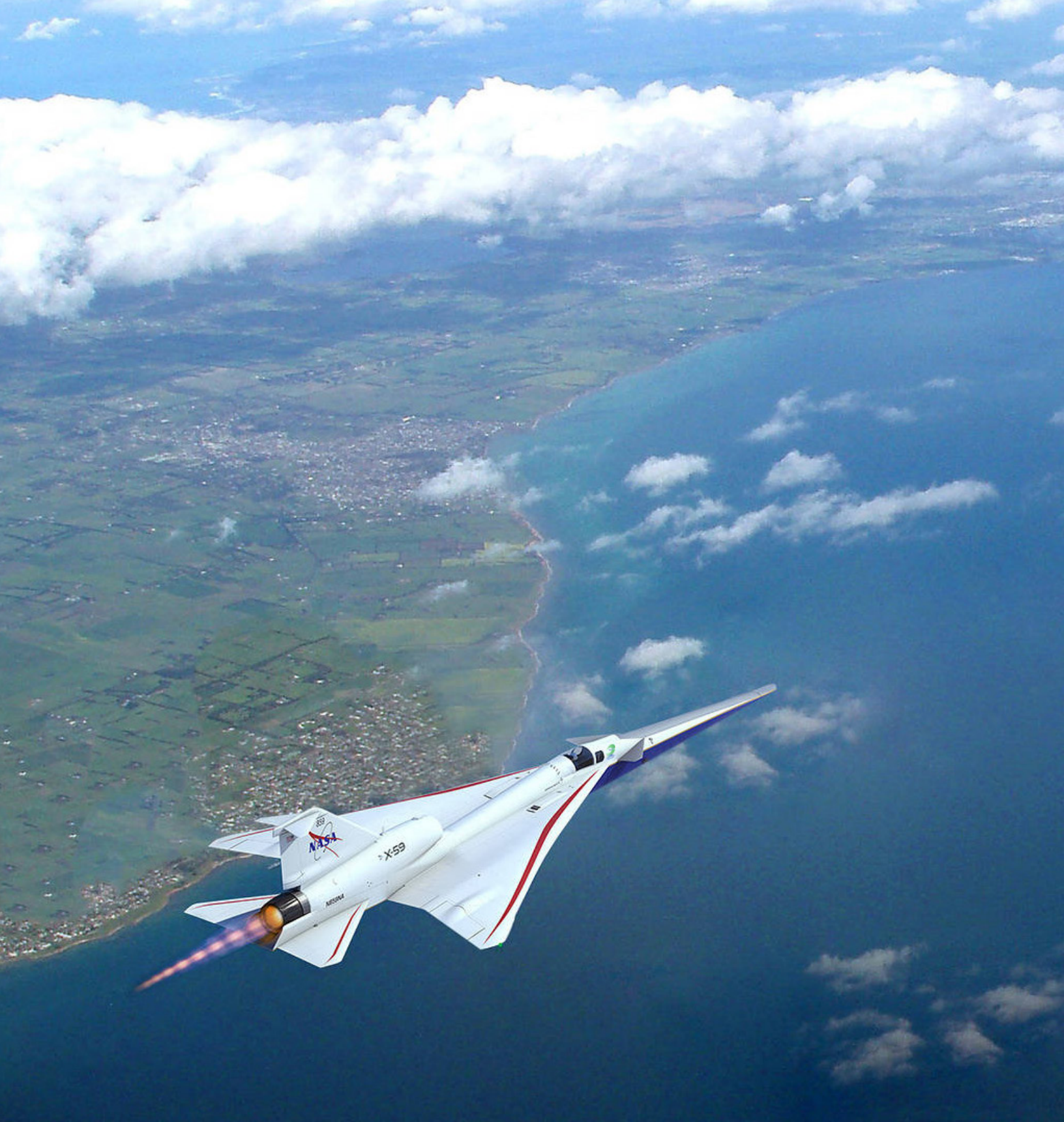
NASA's X-59, seen here in this Lockheed Martin illustration, is the centerpiece of the Quesst mission that could make supersonic flight over land possible, dramatically reducing travel time in the United States or anywhere in the world. The X-59 is designed to reduce the loudness of a sonic boom to a gentle thump to people on the ground. It will be flown over select U.S. communities to gather data on human responses to the sound generated during supersonic flight and deliver that data set to U.S. and international regulators. Credit: Lockheed Martin
