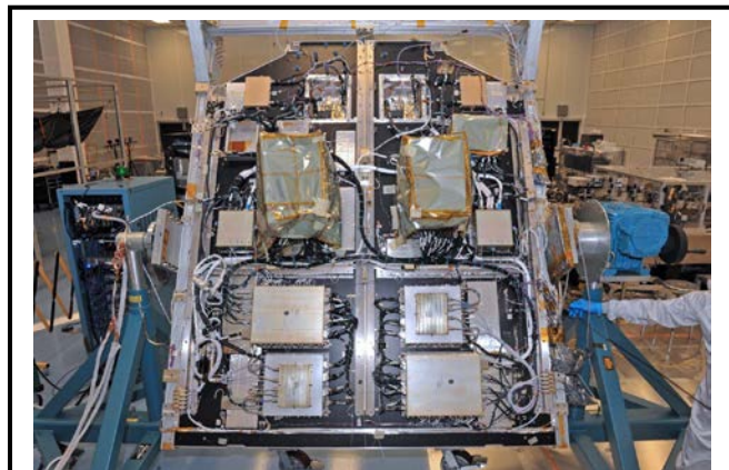
The Laser Communications Relay Demonstration (LCRD) payload, shown here, is completed and in storage in the clean room at NASA Goddard Space Flight Center. Scheduled to launch in 2020, LCRD will simulate communications support after validating optical communications for two years with a test payload on the International Space Station and two dedicated ground stations in California and Hawaii.
