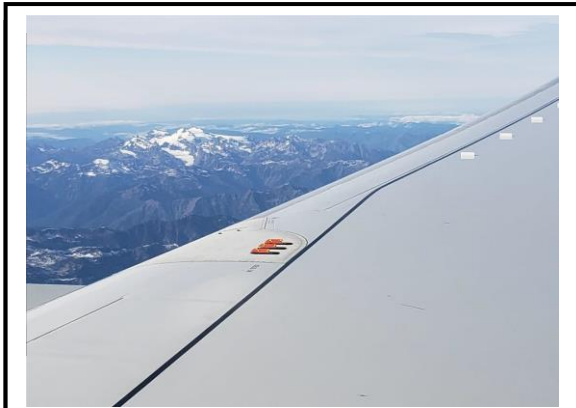
The picture above captures a flight test of a NASA system that automatically deploys and retracts small wing vanes known as vortex generators needed for takeoff and landing. The system uses NASA-developed materials that change shape in response to changes in temperature.
