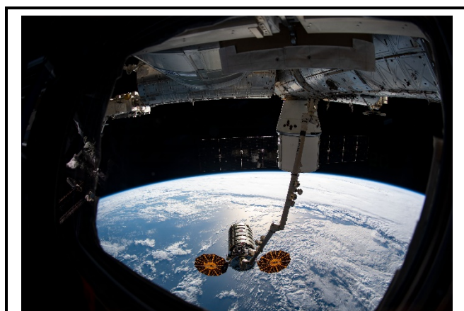
The Northrop Grumman Cygnus resupply spacecraft is shown grappled by the Canadarm2 robotic arm following its detachment from the Unity module and just before release. Behind the robotic arm, the SpaceX Dragon is seen still attached to the ISS Unity module (August 6, 2019).
