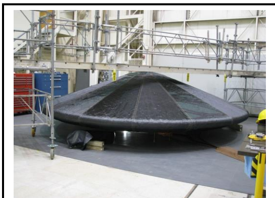
The LOFTID Engineering Design Unit of the Aeroshell is seen here at Langley Research Center (LaRC) undergoing mass property testing. The LOFTID project aims to advance hypersonic inflatable aerodynamic decelerator technology by performing orbital velocity atmospheric entry experiment.
