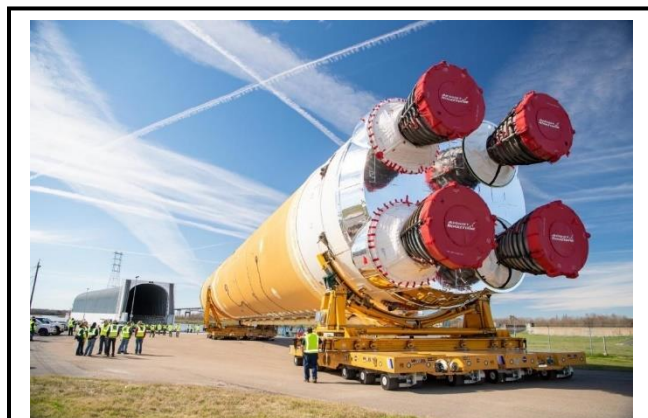
Engineers and technicians completed installation of all four RS-25 engines, shown above, that will provide the necessary thrust for the SLS rocket to reach space. This installation completes core stage assembly. The core stage is now at SSC preparing for Green Run testing.
