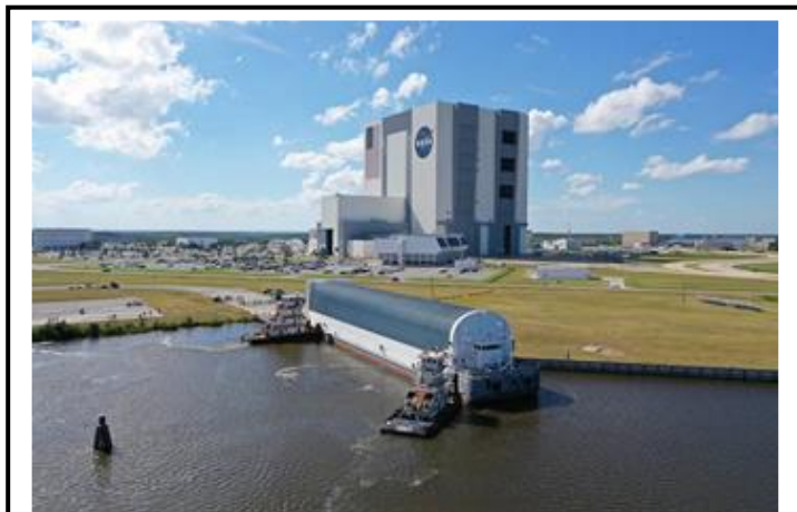
NASA's Pegasus Barge is shown here arriving at the Launch Complex 39 turn basin wharf at Kennedy Space Center (KSC) in Florida to make its first delivery to KSC in support of the Agency's Artemis missions. The upgraded 310-foot-long barge arrived September 27, 2019, ferrying the 212-foot-long Space Launch System (SLS) rocket core stage pathfinder. Weighing 228,000 pounds, the pathfinder is a full-scale mock-up of the rocket's core stage and will be used to validate ground support equipment and demonstrate it can be integrated with KSC facilities.
