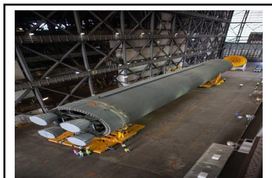
This image shows the Space Launch System (SLS) 212-foot-long core stage pathfinder at the north end of the transfer aisle inside the Vehicle Assembly Building (VAB) at Kennedy Space Center (KSC). The Exploration Ground System (EGS) is using the core stage pathfinder to practice offloading, moving and stacking maneuvers, using important ground support equipment to train employees and certify all the equipment works properly.
