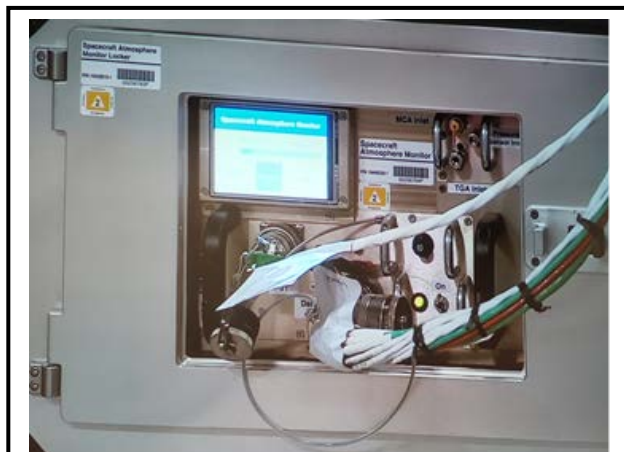
The Spacecraft Atmosphere Monitor (SAM), shown here, was launched to the International Space Station (ISS) and has begun operating successfully.
