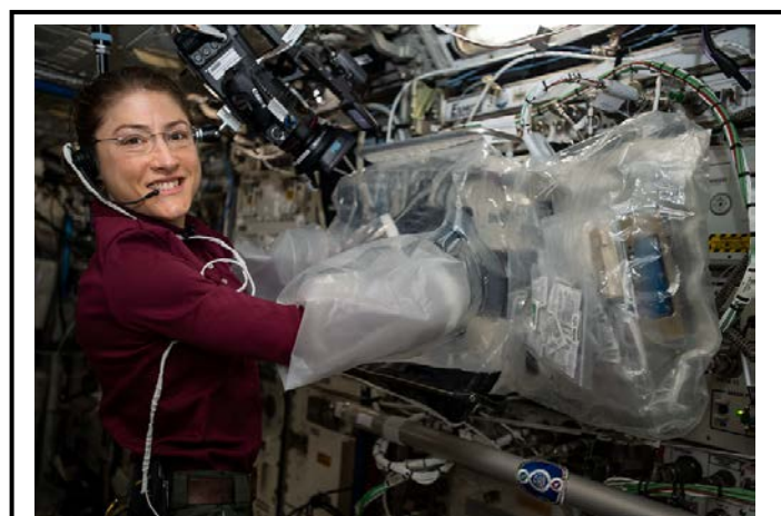
Expedition 60 Flight Engineer Christina Koch (NASA) is shown here activating the new BioFabrication Facility to test its ability to print cells on August 2, 2019. Researchers are exploring whether the weightless environment of space may support the fabrication of human organs in space. An incubator houses the tissue samples to promote cohesive cellular growth over several weeks. Earth's gravity inhibits 3-D bioprinters and incubators from recreating and growing complex organic structures.
