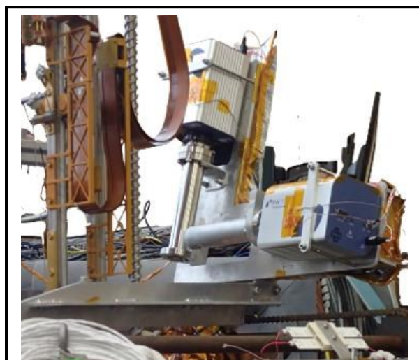
To enable In-Situ Resources Utilization, the Polar Resources Ice Mining Experiment project will deliver water-enriched lunar regolith for identification and quantification of water during an experiment on an early Commercial Lunar Payload Services (CLPS) lander. The Regolith and Ice Drill for Exploring New Terrain are shown above.
