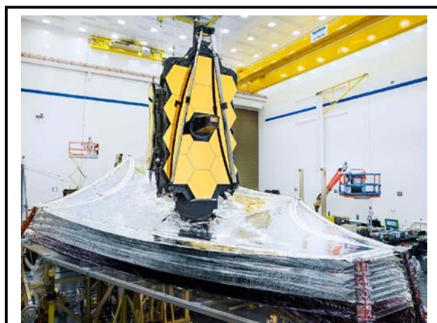
Image depicting the deployment and tension of the five-layer sunshield, which will protect the James Webb Space Telescope once it is in orbit.
