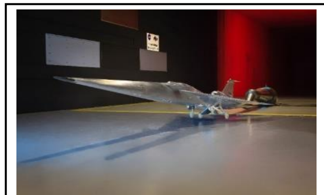
Pictured is the Quiet Supersonic Technology (QueSST) vehicle during a Ground Effects Test at the Langley Research Center (LaRC) 14-foot by 22-foot Subsonic Wind Tunnel.
