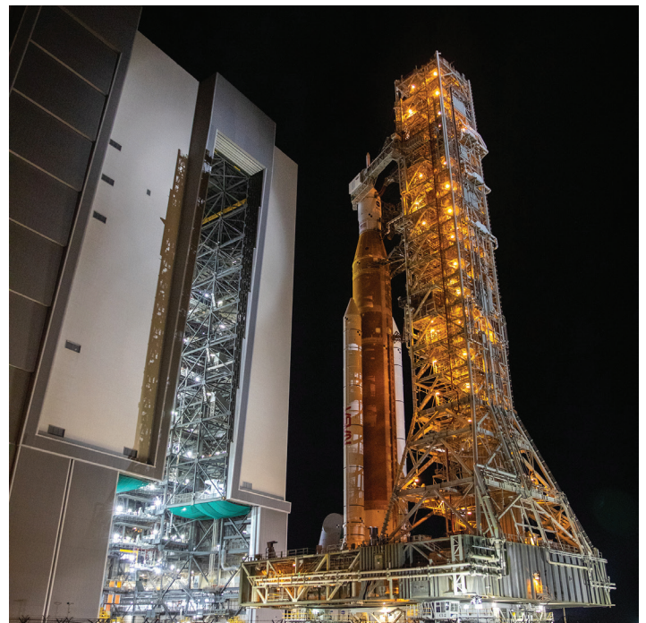
The nearly 400-foot-tall mobile launcher, atop crawler-transporter 2, with NASA’s Space Launch System rocket and Orion spacecraft atop, rolls out of the Vehicle Assembly Building’s High Bay 3 to begin its journey to Kennedy’s Launch Pad 39B ahead of the Artemis I mission on Nov. 4, 2022. The first in a series of increasingly complex missions, Artemis I was the first integrated test of the agency’s deep space exploration systems. Through Artemis missions, NASA will establish a long-term lunar presence for scientific discovery and prepare for human missions to Mars. NASA/Isaac Watson
