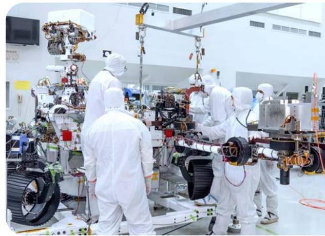
Engineers install the robotic arm on the Perseverance rover.
