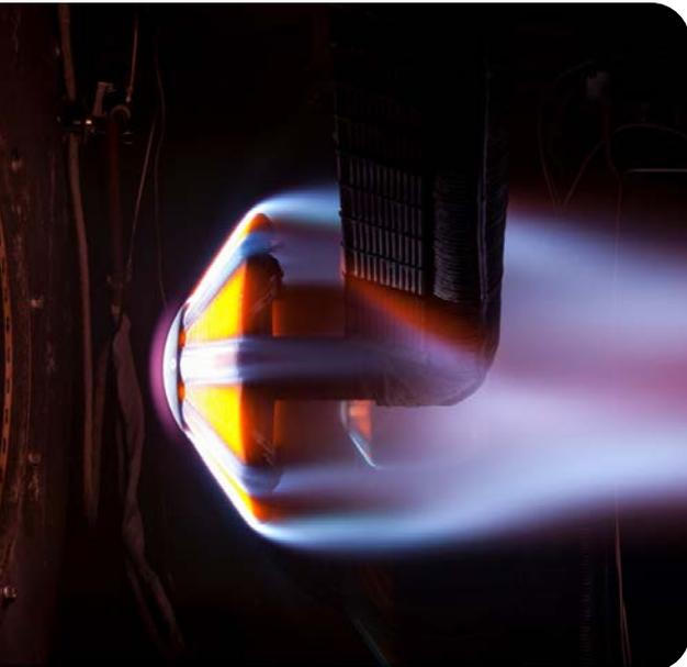
Prototype test at Ames Research Center's Arc Jet Complex
