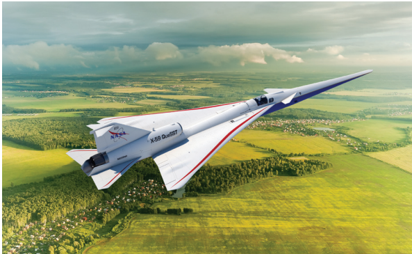
Artist concept of the X-59 QueSST flying over a U.S. community where residents will be asked to share their perceptions of the airplane's quieter sonic booms—if they hear anything at all. Ground-based sensors also will measure sound levels. Credit: NASA
