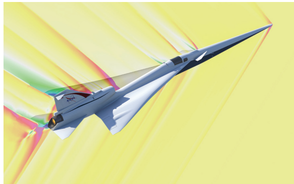
This computer simulation shows how shockwaves move away from the X-59 as it flies faster than sound. The pattern is different from the way shockwaves from a conventional supersonic aircraft come together to produce a sonic boom. Instead, the X-59 will produce a quieter sonic thump. Credit: NASA
