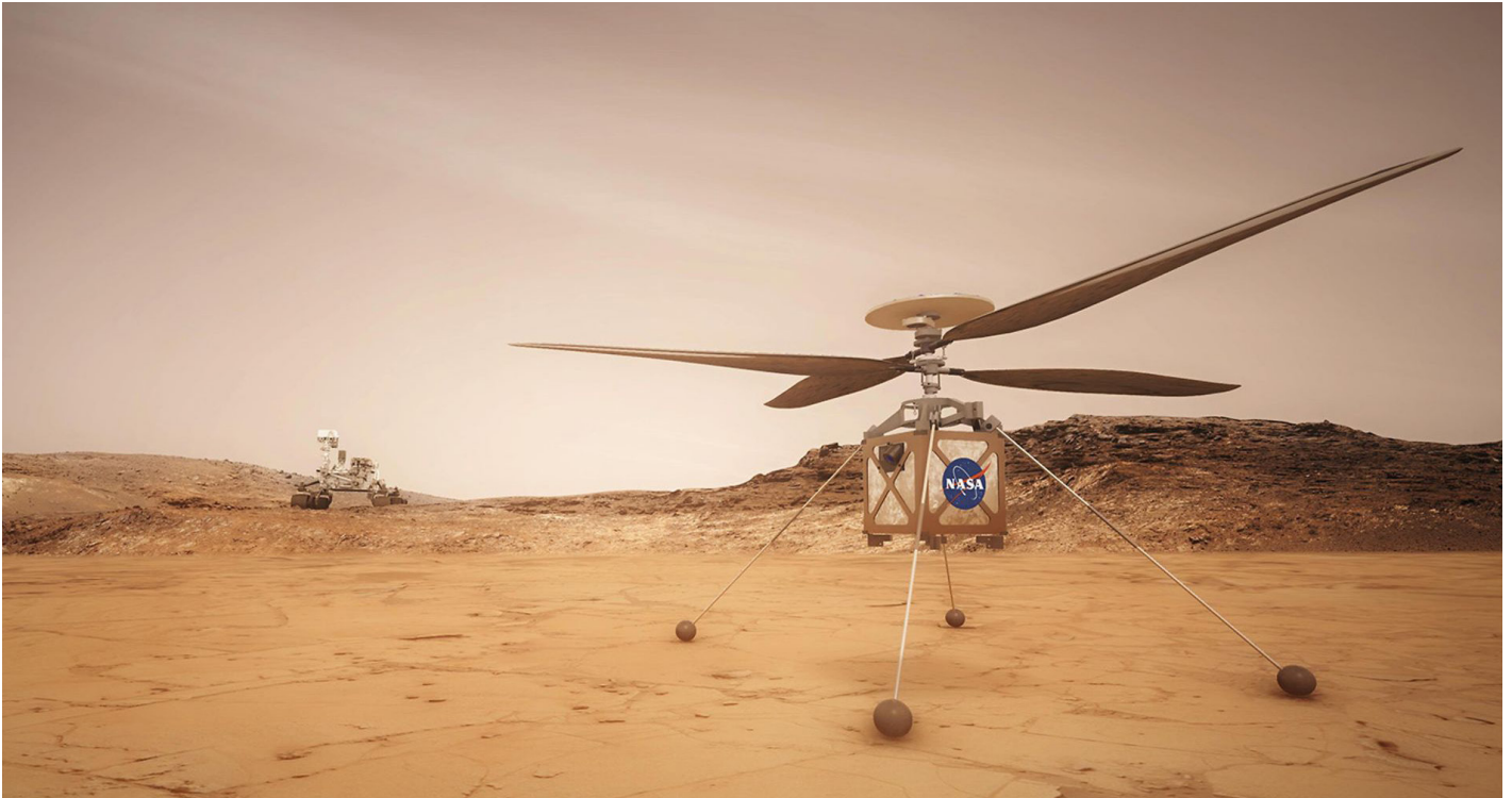
Figure 13. Ingenuity has long rotor blades because of the thin Martian atmosphere. Credit: NASA
