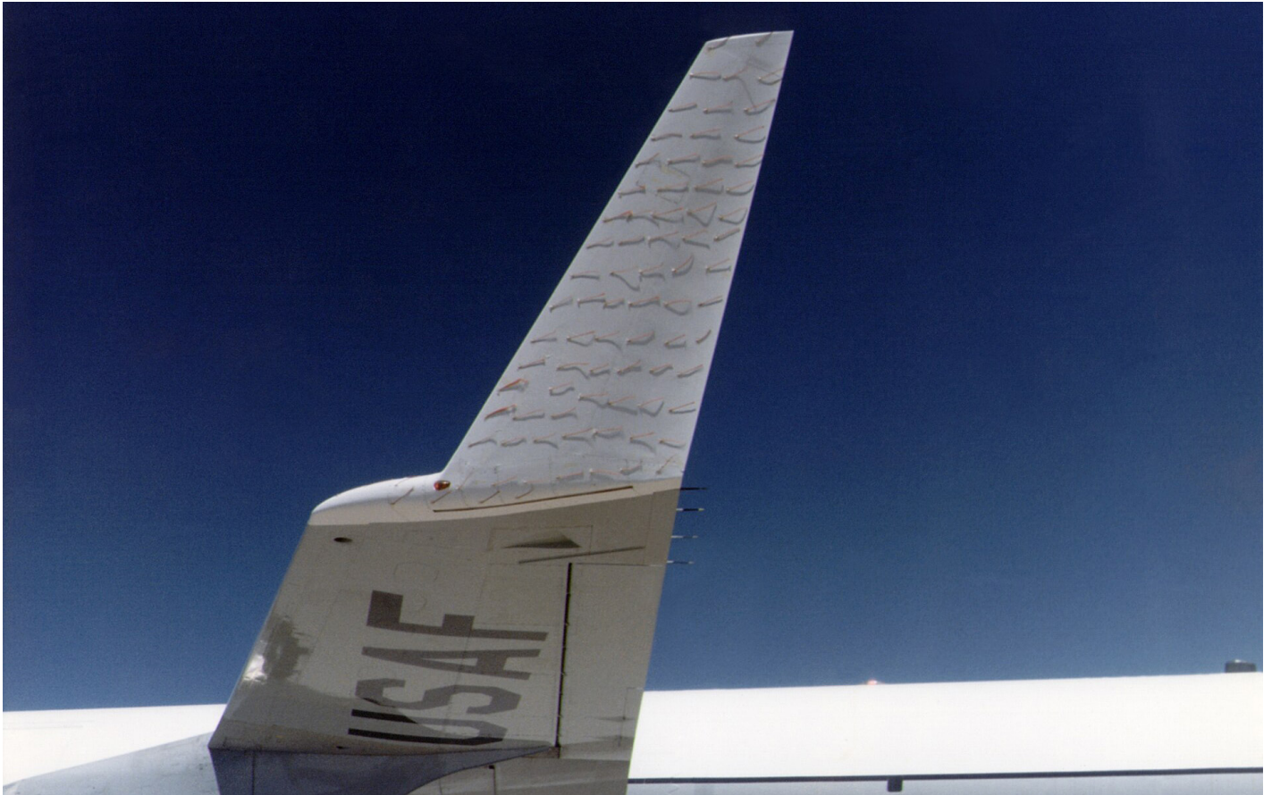
Figure 8. Winglets help reduce air vortexes.
