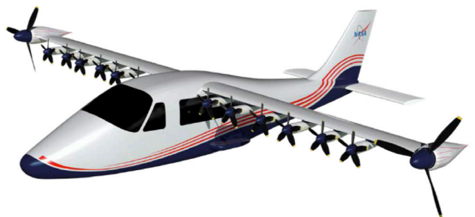
Figure 1. NASA's X-57 is powered completely by batteries in order to reduce harmful emissions.
