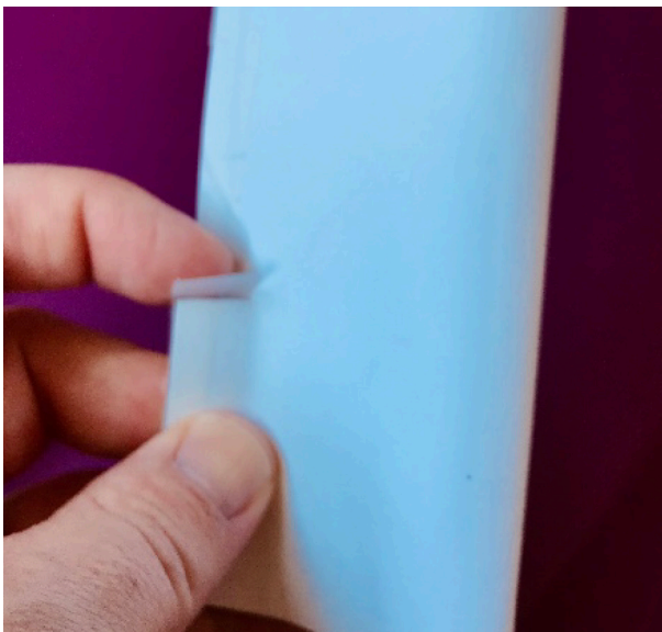
Figure 4: Tape both ends of each aileron.
