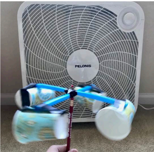
Figure 4: Place the anemometer in a stream of air to see it rotate.
