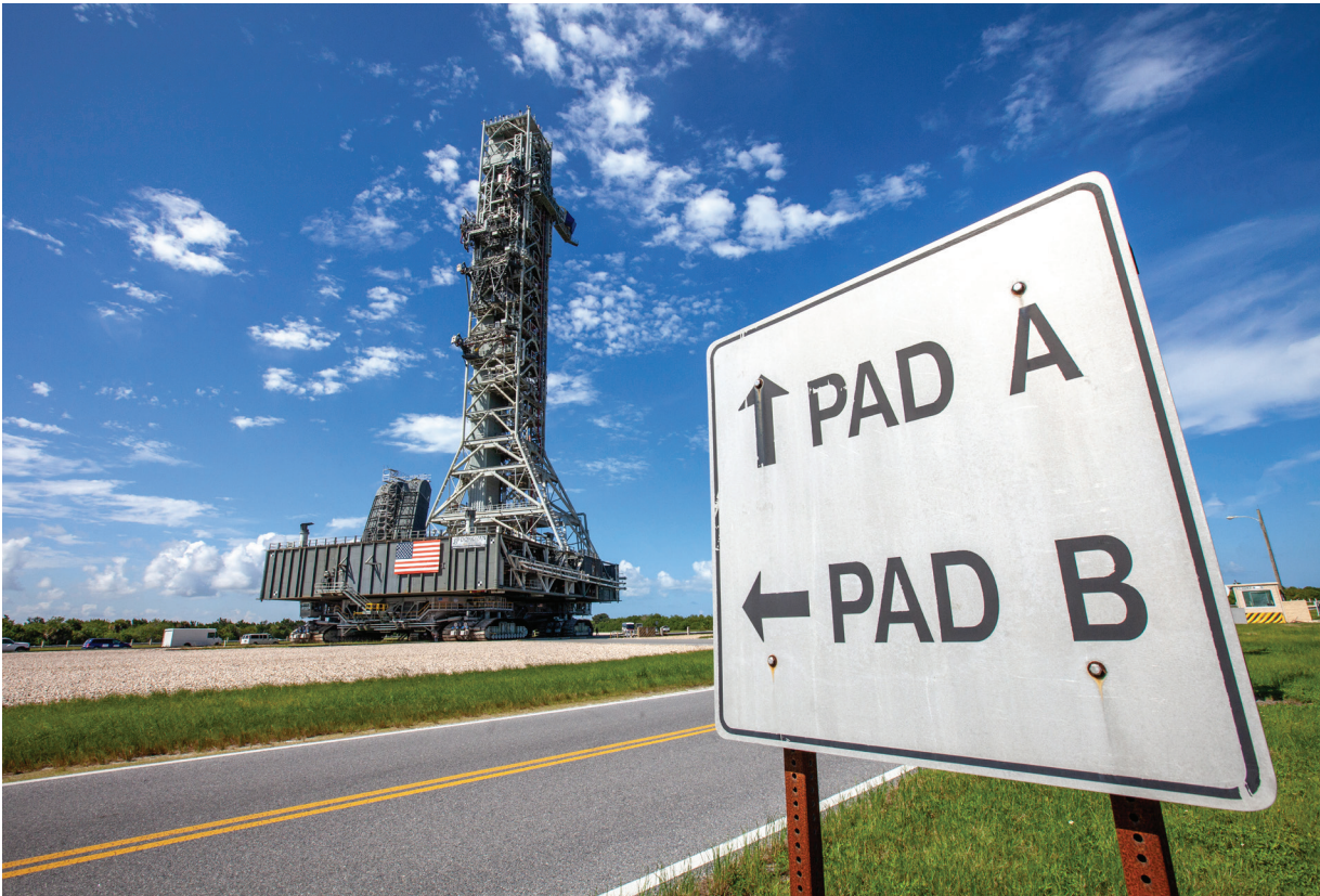
NASA's mobile launcher (ML) atop crawler-transporter 2 moves along the crawlerway and nears the turn to Launch Pad 39B on Sept. 10, 2019 at NASA's Kennedy Space Center in Florida. NASA's Exploration Ground Systems moved the mobile launcher to the launch pad, where teams will complete testing and checkout on the launcher for the Artemis I mission. Photo credit: NASA/Ben Smegelsky
