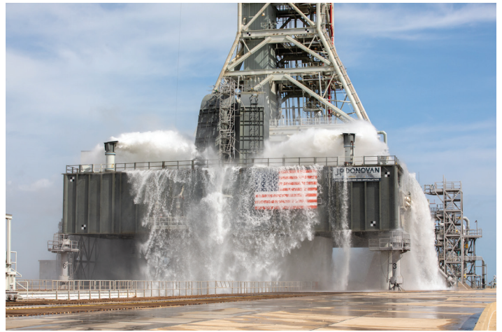
A wet flow test at Launch Pad 39B on September 13, 2019, tested the sound suppression system that will be used for launch of NASA's Space Launch System for the Artemis I mission. During the test, about 450,000 gallons of water poured onto the Pad B flame deflector, the mobile launcher flame hole and onto the launcher's blast deck. Photo credit: NASA/Kim Shiflett
