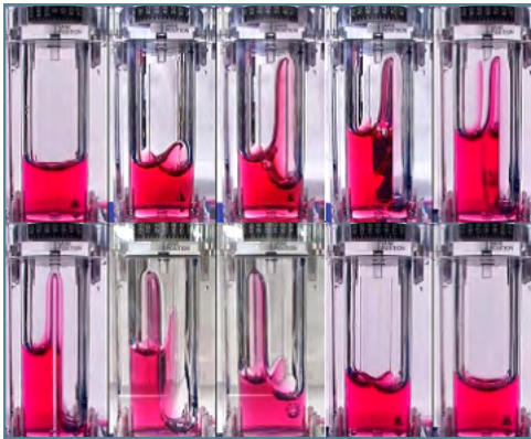
Figure 17. Equilibrium interfaces for Vane Gap-1 for several vane dial angles: 0, 36, 43, 53, 59.5, 90, 127.5, 134.5, 150.5, 180 degrees (from top left to bottom right).
