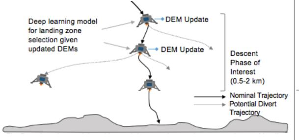
Fig. Deep learning model enables real-time terrain mapping, processing, and landing zone selection/divert decision making given digital elevation maps (DEMs).
