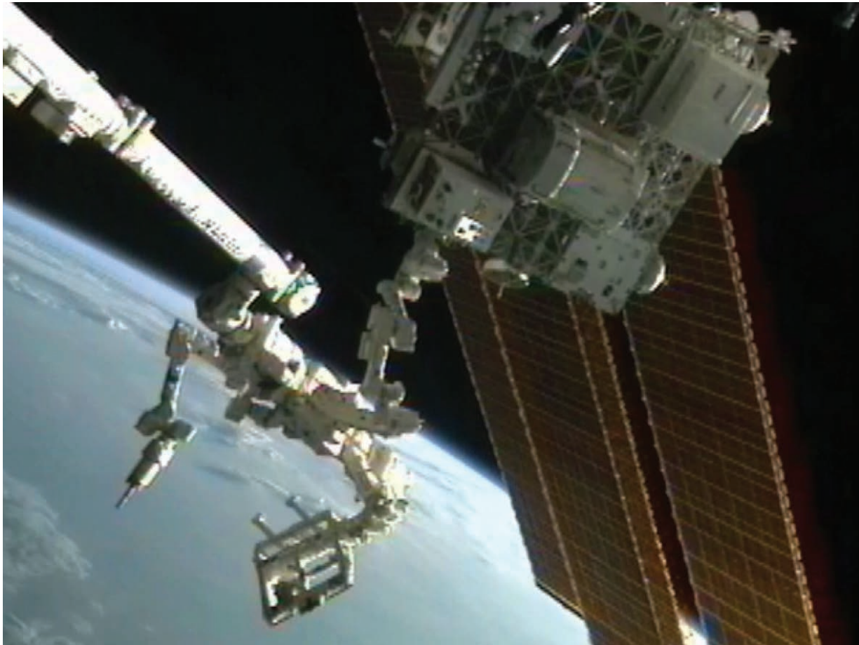
The RRM investigation (center, on platform) uses Canadarm2, the ISS robotic arm, and the Canadian Dextre robot (right) to demonstrate satellite-servicing tasks.
