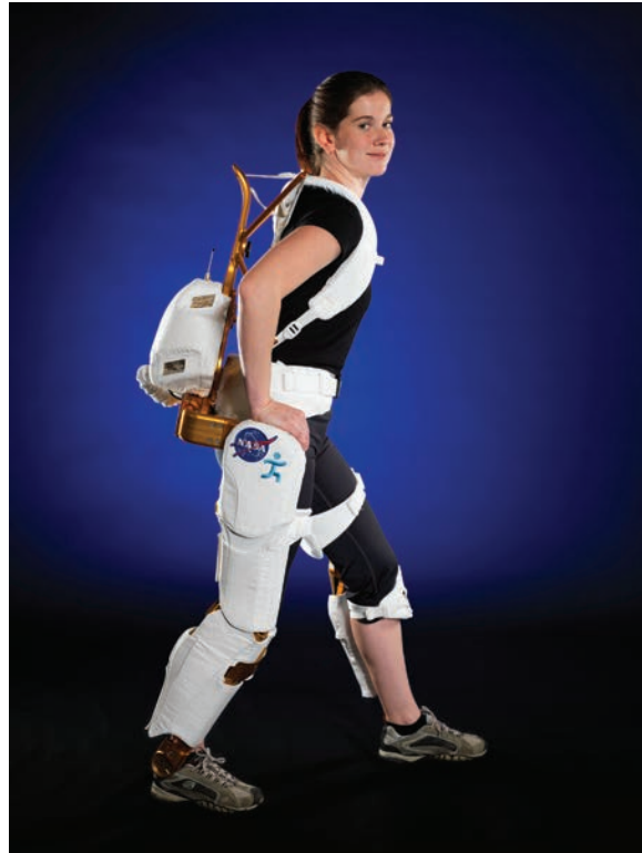
NASA Project Engineer Shelley Rea demonstrates the X1 Robotic Exoskeleton, which could improve the mobility and strength of astronauts and paraplegics.
