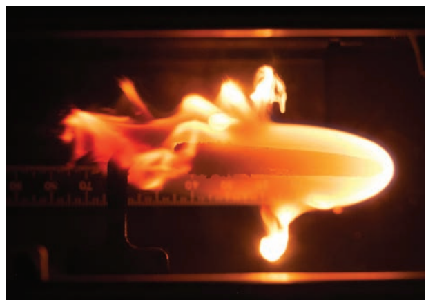
Image taken during a BASS-II (Burning and Suppression of Solids - II) experiment flame test.
