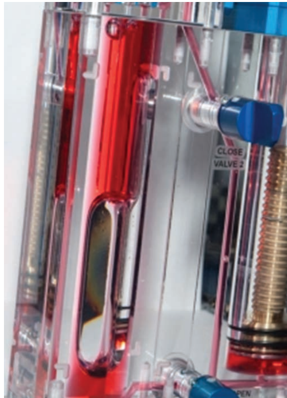
A view of Capillary Flow Experiment-2 Interior Corner Flow 3 vessels set up during an experiment aboard the ISS. This study looks at capillary flow in interior corners.
