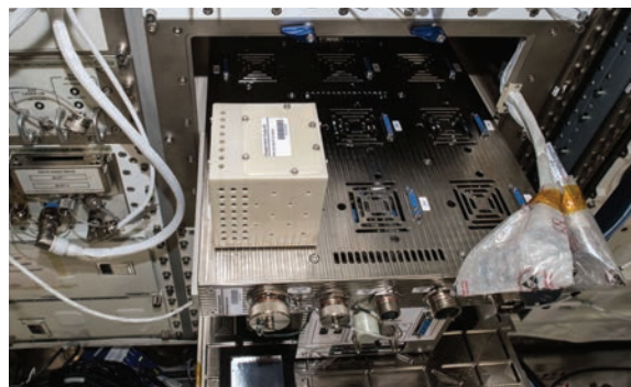
The ICE Cubes Facility located in the Columbus European Physiology Module rack is a capable experiment platform that offers flexibility to host many different experiments in the CubeLab form factor. Pictured is the first experiment module hosted in the facility (taken June 5, 2018).
