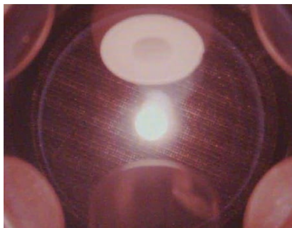
Molten alumina levitating in the center of six electrodes onboard the ISS. Image credit: JAXA
