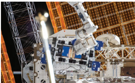
View of the MISSE-FF taken by the External High Definition Camera on April, 19 2018. The MISSE-FF platform provides the ability to test materials, coatings, and components or other larger experiments in the harsh environment of space.
