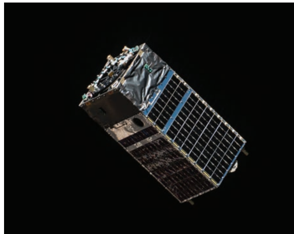
The Kestrel Eye IIM (KE2M) CubeSat is pictured shortly after it was deployed from the tip of the Dextre attached to the Mobile Servicing System on October 24, 2017. The KE2M is carrying an optical imaging system payload that is being used to validate the concept of using microsatellites in LEO to support critical operations.
