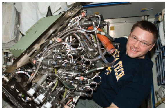
NASA astronaut Douglas H. Wheelock, Expedition 25 commander, is photographed with the Sabatier Assembly—just prior to installation into Oxygen Generator System rack. Image credit: NASA
