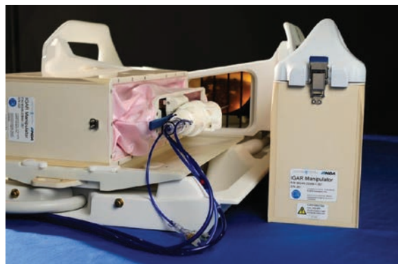
IGAR manipulator and full breast intervention platform mounted on the patient support structure with a biopsy tool attached.
