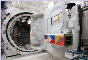
BIRDS-2 deployed from the Japanese Experiment Module (JEM). From left to right: JEM airlock slide table with BIRDS-2 CubeSats representing Bhutan, Malaysia, and the Philippines, ready for deployment (July 30, 2018); BIRDS-2 satellite deployment from the JEM Small Satellite Orbital Deployer (August 10, 2018); BIRDS-2 satellites following deployment.
