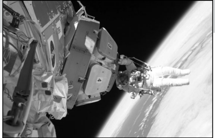
An astronaut installs the Cupola to Tranquility Node.
