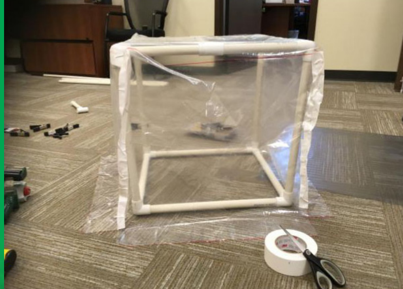
Figure 12. Step 6 of Classroom VEGGIE assembly: Attach modified shower curtain to PVC frame (as described above).
