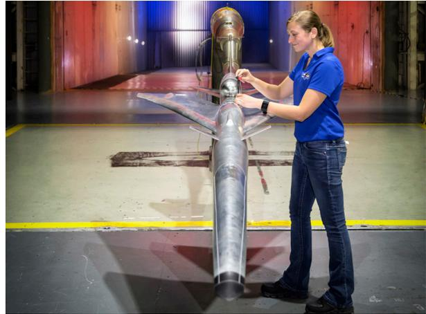
Figure 2. Test Engineer Samantha O'Flaherty finalizes the set-up of the Quiet Supersonic Technology (QueSST) Preliminary Design Model inside the 14- by 22-foot subsonic wind tunnel at the NASA Langley Research Center.
