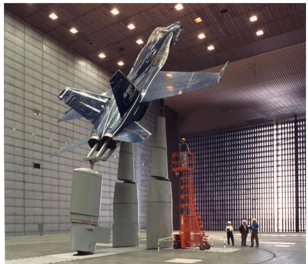
Figure 3. An F/A-18 fighter aircraft in the giant 80- by 120-foot wind tunnel at the NASA Ames Research Center.
