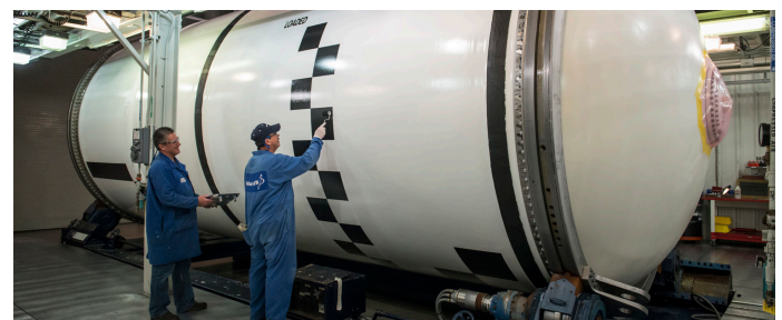
EM-1 Solid Rocket Booster Segment
