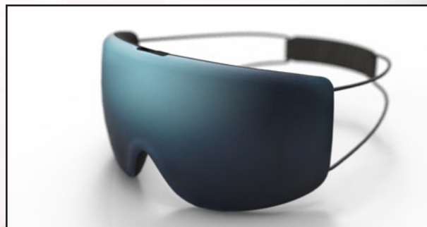
LumosTech wearable technology is a sleep mask to help circadian alignment by emitting short light pulses.
