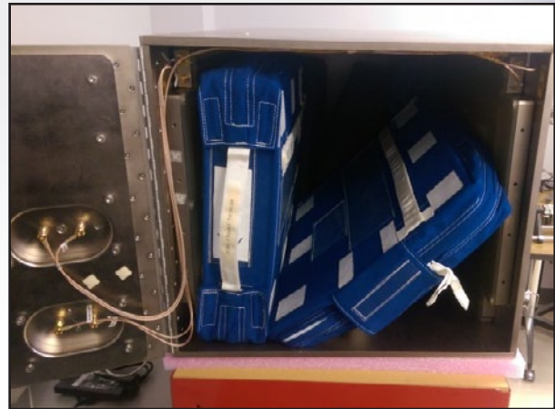
Sensors inside the locker detect RFID tags on items in medical kits. When items are removed, the inventory is updated.
