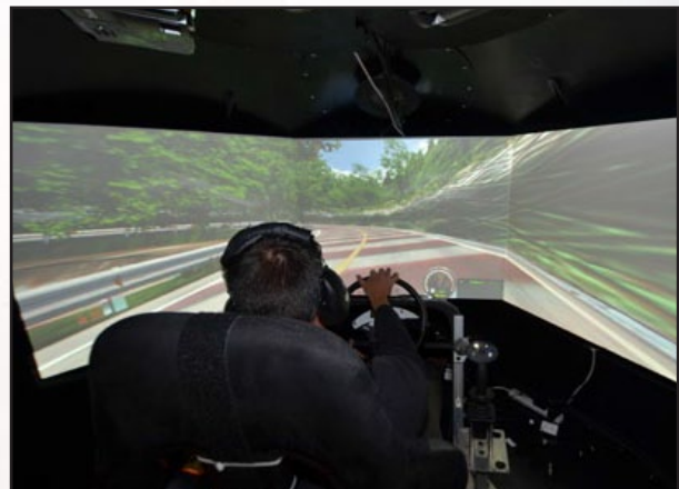
A test subject attempts to maintain lane position on a twisting road. The Manual Control study assessed complex sensorimotor tasks such as landing a spacecraft or operating a rover.
