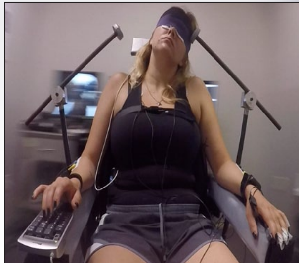
Rotating chair simulates Orion re-entry while subject uses a keypad for tests of manual dexterity and mental arithmetic.
