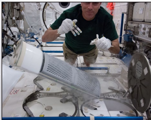
An ISS crewmember adds blood samples to the Minus Eighty-degree Laboratory Freezer for the ISS (MELFI) for storage prior to return to Earth for analysis. ISSMP provides essential logistic support to expedite the return of these samples to PIs.
