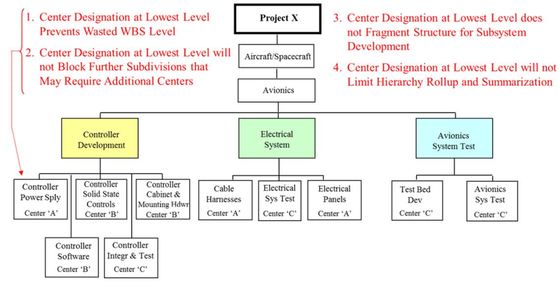
**Figure 3-17: Center Breakout Guidance for a WBS**
