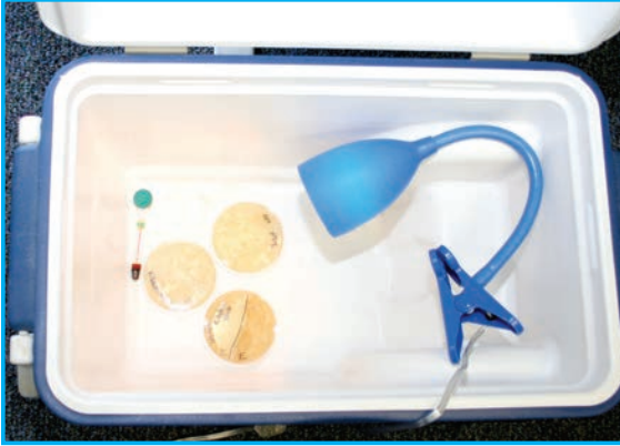
Image 1: Incubator made from a hard-side cooler.
