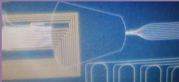
Images of photonic circuits: the blue lines are photonic integrated waveguides, while the yellow lines are metal lines for integrated heaters.
