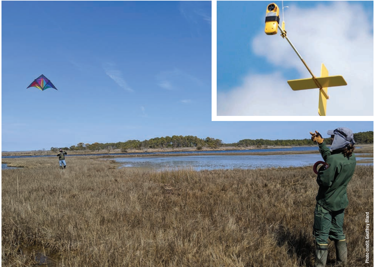
The Aeropod (inset), shown here being launched with a kite near Wallops Flight Facility, is a stabilized, suspended platform for Earth observations.
