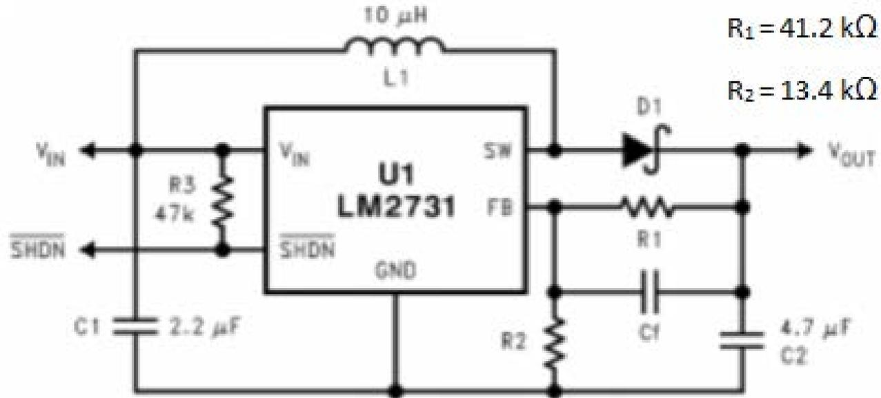
Figure 1: LM2731 Basic Application Circuit
