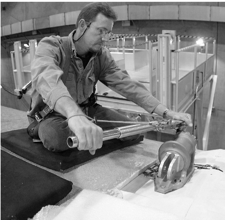
A technician torques bolt fasteners on the redesigned -Y bipod fitting on ET-120 at NASA's Michoud Assembly Facility in New Orleans in November 2004. The bipod redesign was one of the Return to Flight changes to the external tank to minimize potential debris by eliminating the large insulating foam covering the bipod area in favor of electric heaters. (Photo credit: Lockheed Martin)
