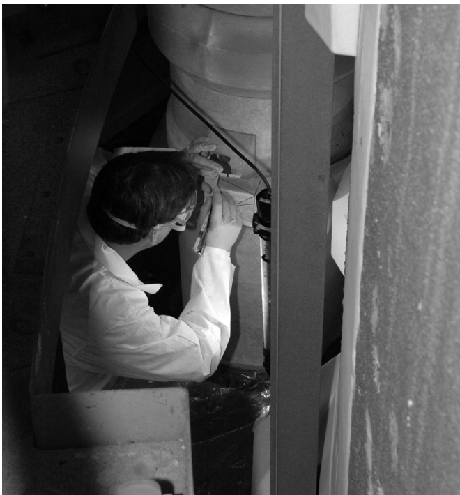
A technician at the Kennedy Space Center maps out the cutting area of the liquid oxygen (LO2) feedline bracket where foam insulation and super lightweight ablator, or SLA, cork insulation were removed. Foam insulation was then reapplied without the SLA. (Photo credit: NASA/KSC)
