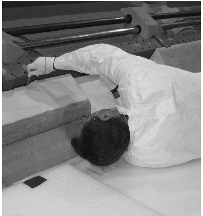
A technician measures foam prior to removing it from ET-120's liquid hydrogen tank protuberance airloads (PAL) ramp in November 2005. Following STS-114, studies and testing determined that both the liquid oxygen and the liquid hydrogen PAL ramps could be removed from the external tank to minimize potential foam loss. The two PAL ramps, made entirely of foam, weighed almost 37 pounds. ET-119 was the first tank to fly without PAL ramps. (Photo credit: Lockheed Martin)
