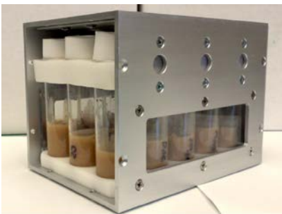
Figure 14a: The vial assembly slides into the ventilated metal shell that allows for even temperature distribution within the SABL unit.
