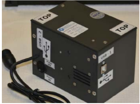
Figure 13b. The integrated AFEx payload was about 10 x 10 x 15 cm in size and utilized external power.
