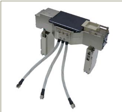
Figure 7: The stand-alone CU configuration showing cable connectors and removable SSD on the top.
