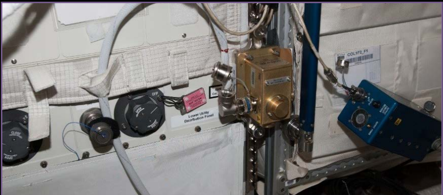
SAMS Sensor (SE-F02) supporting science operations near the European Drawer Rack in the Columbus Module. (Image credit: NASA)
