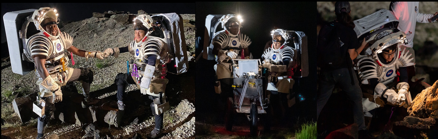
The Joint Extravehicular Activity and Human Surface Mobility Program Test Team (JETT) testing tools and spacesuits in a rock yard at NASA's Johnson Space Center, simulating the uneven terrain of the lunar surface, in preparation for Moonwalks
