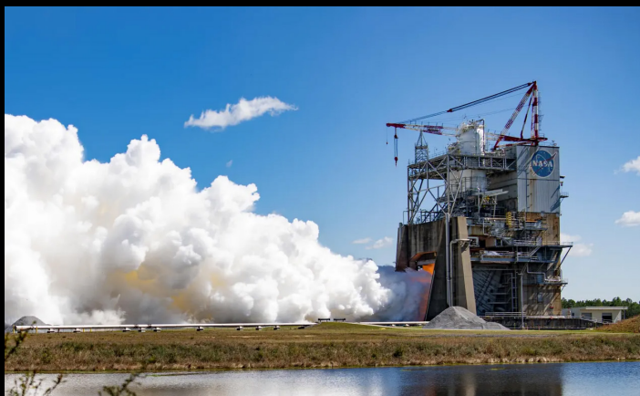
Certification testing for production of new RS-25 Retrofit 3b engines to power the SLS rocket, beginning with Artemis V, completed early April 2024
