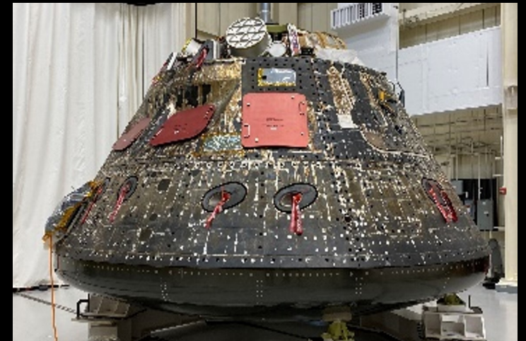
Orion environmental test article being prepared for vibro-acoustic testing at NASA's Neil Armstrong Test Facility
