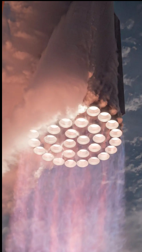
March 14, 2024—For the second time, all 33 Raptor engines on the Super Heavy Booster started up successfully and completed a full-duration burn during ascent. Credit: SpaceX
