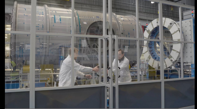
Engineers at Thales Alenia Space Italia gently guide HALO from its welding platform to an integration test stand.
