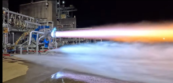
Blue Origin's BE-7 team conducted a successful Thrust Chamber Assembly test at NASA Marshall Space Flight Center.
