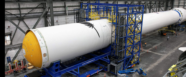
The first and second stages of New Glenn's test vehicle mated for the first time enabled Blue Origin to exercise their tooling and stage interfaces in preparation for the first launch.
