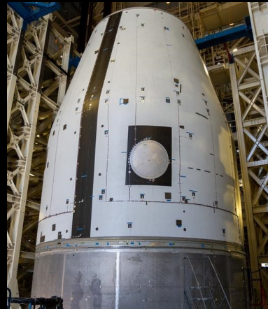
Artemis IV universal stage adapter development test article at Marshall for testing
