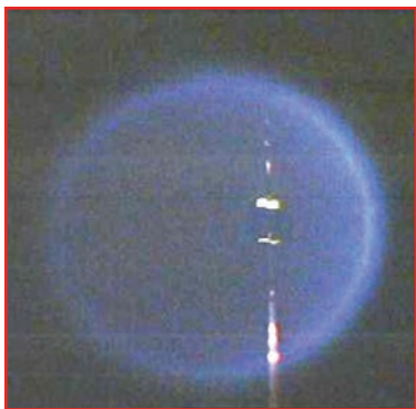
Figure 2. Flame image of n -heptane droplet burning in 70 percent carbon dioxide, 21 percent oxygen, balance nitrogen and translated to the right at 3 cm/s. (Image credit: NASA, FLEX experiment)
