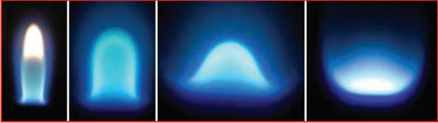
Figure 5. Effect of increasing coflow velocity (from left to right, where the image scale is not consistent) on lifted flame behavior from exploratory tests for the Structure & Liftoff In Combustion experiment, which were conducted in 2009 on the ISS as part of the Smoke Point In Coflow experiment.
