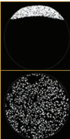
Figure 15. Top: An Earth-based experiment, shows an agglomeration of tin particles (white) that rose to the surface because they are lighter than the host lead-tin liquid. Bottom: With buoyancy forces minimized in a microgravity environment, a reasonably uniform dispersion of tin particles in the liquid was maintained. Image courtesy of J. Alkemper, V. Snyder and P.W. Voorhees, Northwestern University.
