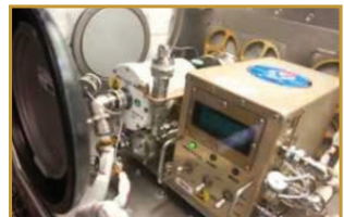
Figure 8. Left: The Coarsening of Solid-Liquid Mixtures Sample Processing Unit. Right: The Electronics Control Unit.
