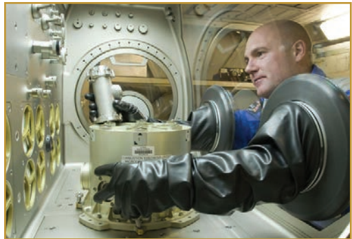
Figure 7. Left: The Microgravity Science Glovebox Rack on ISS. Right: A view of the working volume of the MSG.
