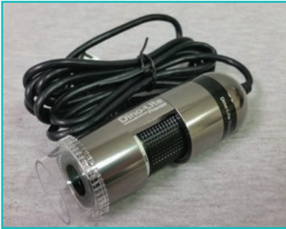
NanoRacks Microscope-3 is an off-the-shelf USB microscope. Image is courtesy of NanoRacks LLC.
