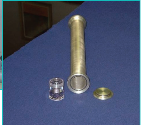
The Enhanced Diffusion-Controlled Crystallization Apparatus for Microgravity Image Courtesy of NASA's Marshall Space Flight Center.
