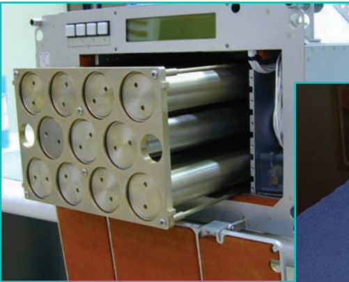
The Enhanced Diffusion-Controlled Crystallization Apparatus for Microgravity Image Courtesy of NASA's Marshall Space Flight Center.
