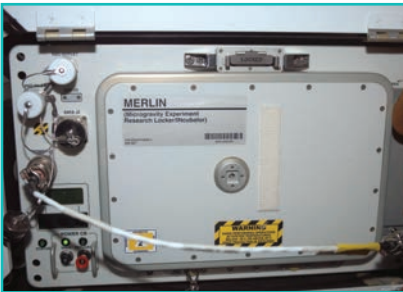
View of Microgravity Experiment Research Locker/Incubator on the forward middeck on Space Shuttle Endeavour. Photo was taken during STS-123 / Expedition 16 joint operations.
