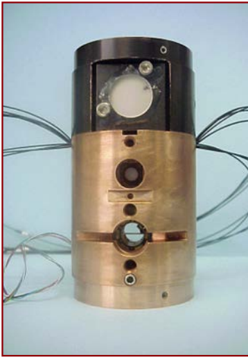
Figure.5.4.1. Pictured is a DEvice for the Study of Critical Liquids and Crystallization Alice Like Insert sample cell. (Source: Y. Garrabos)
