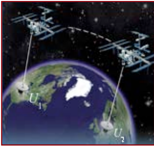
Figure 4.2.1. Schematic of ACES global time transfer comparison. (Source: Luigi Cacciapuoti, European Space Agency Atomic Clock Ensemble in Space project).
