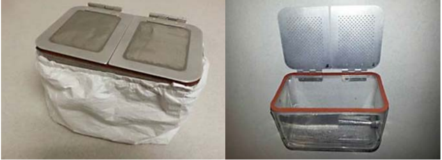
Figure 9. The Mouse Transfer Box (MTB) fits inside the Animal Access Unit for transfer of rodents into/from the Rodent Habitat and is also placed in the Microgravity Science Glovebox for the same purpose. The MTB on the right is shown with the dual lid opened, but it can also be opened half at a time to help sequester animals inside. The MTB on the left is shown with a removable fabric cover in place to provide a more secure environment for animals after they are loaded.
