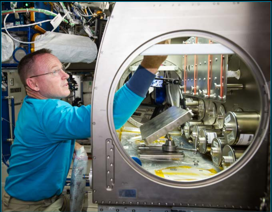
An astronaut performs ISS operations in support of the Rodent Research-1 validation flight in late 2014. The Microgravity Science Glovebox is utilized to receive mice removed from the Animal Access Unit (blue unit in background) after being humanely euthanized. Tissues are harvested, frozen, and transported to Earth for analysis. (Image credit: NASA)
