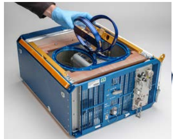
Figure 5. Rodent Habitat. Shown with both access doors open.
