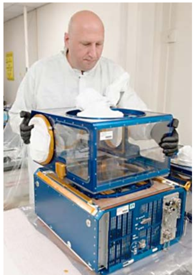
Figure 8. The Animal Access Unit (AAU) is attached during fit check to the top of the Rodent Habitat. The white fabric gloves and gauntlets on the AAU openings are used for animal handling to maintain containment during animal transfers.
