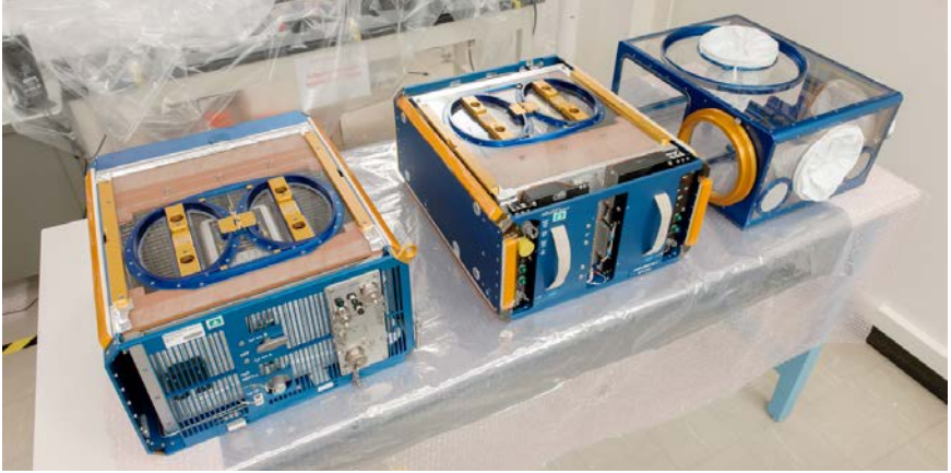
Figure 4. The Rodent Habitat Hardware System. From left: The Rodent Habitat; the Rodent Transporter; and the Animal Access Unit.
