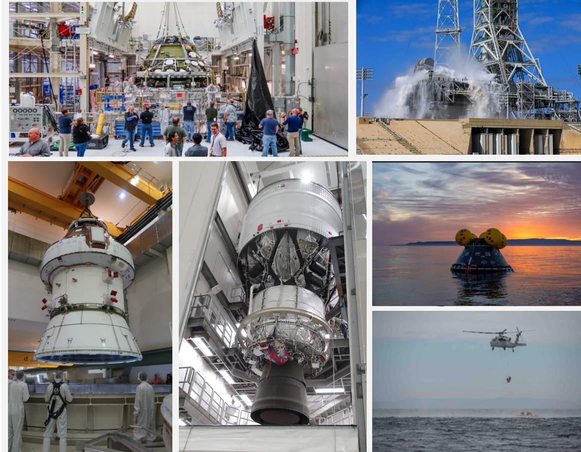
Images (L to R): (1) Artemis II Crew & Service Module; (2) Exploration Ground Systems conducts a water flow test with the mobile launcher; (3) Artemis II spacecraft lifted into Altitude Chamber for EMI/EMC testing; (4) Artemis II ICPS In Storage Cell at ULA DOC at CCSFS; Hardware Acceptance Review complete; (5) Exploration Ground Systems conducts Underway Recovery Test 11
