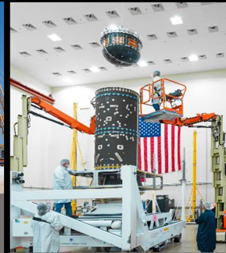
First Xenon tank being installed in the PPE central cylinder. Photo by Maxar Space Systems
