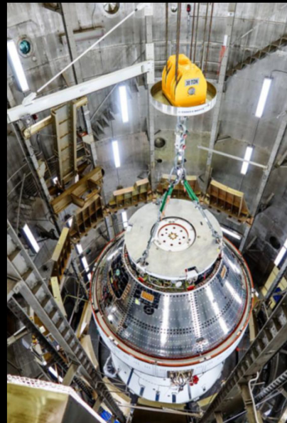
Artemis II Orion spacecraft lifted out of a vacuum chamber after EMI/EMC testing
