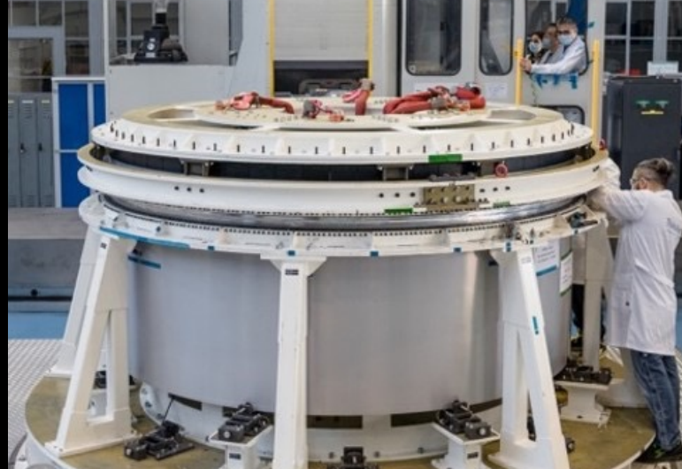
Habitation and Logistics Outpost Primary Structure Assembly
