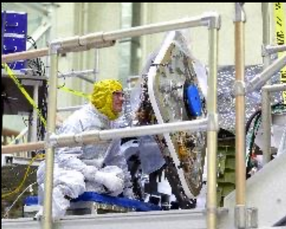
Artemis II Side Hatch in Acceptance Testing
