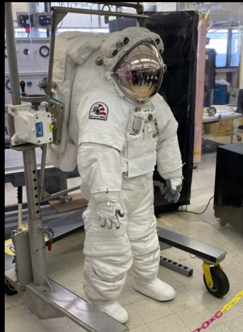
Pressure Testing of NASA's Fully Assembled Exploration Spacesuit
