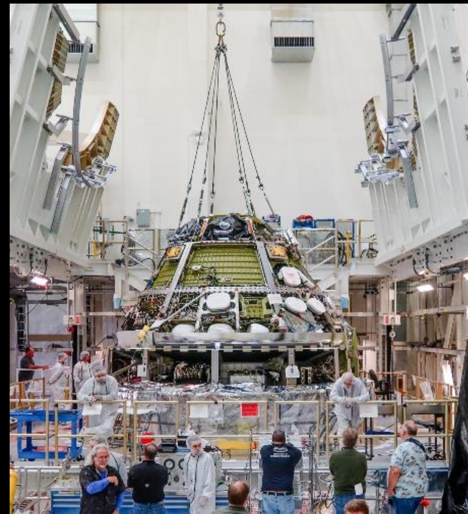
Integration of Crew and Service Modules for the Artemis II Orion Spacecraft Complete
