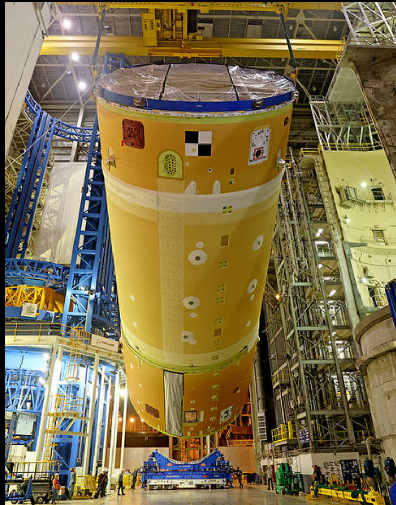
Five Major Structures of the Artemis II Space Launch System Rocket Core Stage are Connected
