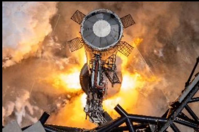
August 20, 2023 — Super Heavy Booster's static fire successfully lit all 33 Raptor engines, with all but two running for the full duration. The test produced approximately 7.9 million lbf of thrust (~3,600 metric tons) and utilized the newly installed Starship flame deflector.
