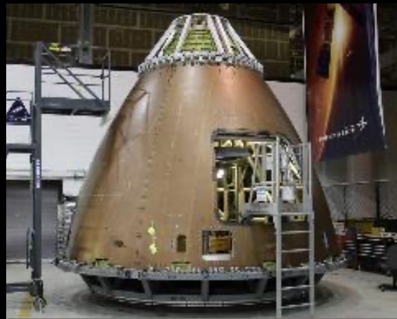
Artemis II Launch Abort System 0 Degree Ogive in Protoqual Testing
