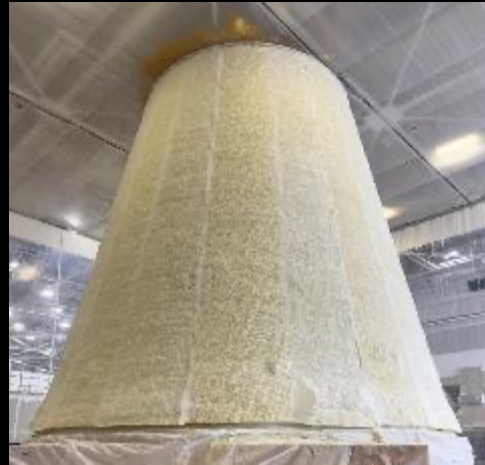
Thermal Protection Applied to Launch Vehicle Stage Adapter
