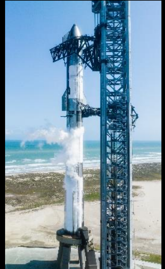
October 24, 2023 - Starship and Super Heavy loaded with more than 10 million pounds of propellant in a flight like rehearsal ahead of second test flight of a fully integrated Starship.
