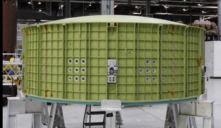
Artemis IV Crew Module Pressure Vessel at Michoud Assembly Facility
