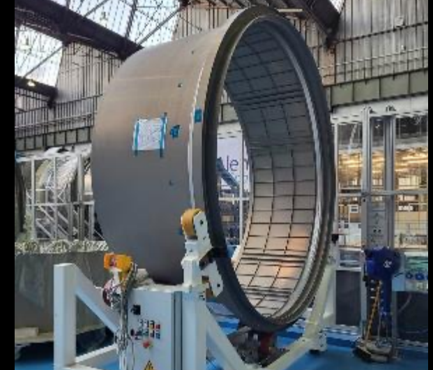
Initial Welds on Gateway I-Hab Primary Structure
