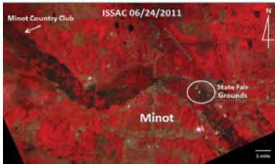
Comparison of Minot, N.D., and Souris River Valley during normal river flow conditions (top image, Landsat Thematic Mapper data) and during flood conditions (bottom image, ISSAC data). Both images have been processed to highlight actively photosynthesizing vegetation in red. Urban areas appear as gray-brown.
