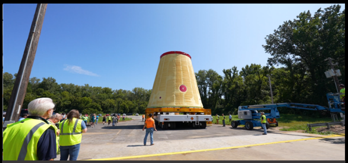
Launch vehicle stage adapter (LVSA), which connects SLS core stage to upper stage, en route to Kennedy
