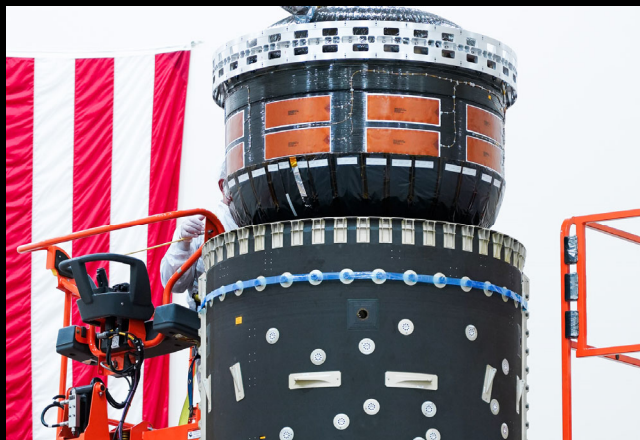
Maxar technicians install xenon tanks into Power and Propulsion Element (PPE) central cylinder for Gateway
