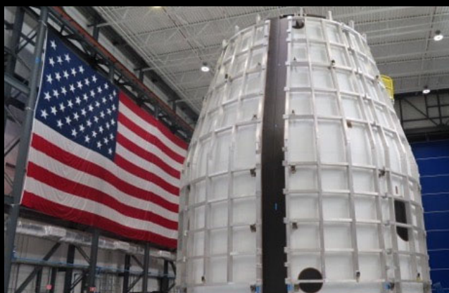
All four universal stage adapter structural qualification article panels are aligned and loaded on Vertical Assembly Tool
