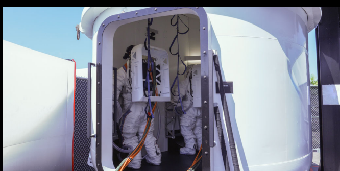
Astronauts in pressurized spacesuits interact with full-scale mock-up of SpaceX Starship HLS airlock
