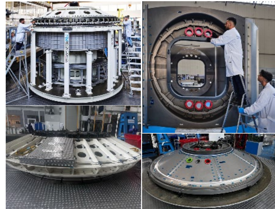
Hab 1 Endcone Welding Progress
